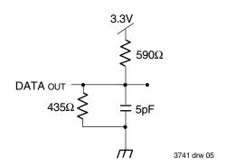
Figure 2. Output Test Load (For thz, tLz, twz and tow)
