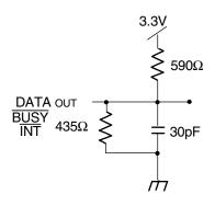
Figure 1. AC Output Test Load
