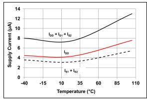
FIGURE 2-12: Sleep State Current vs. Temperature.
