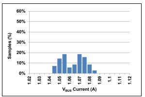
**FIGURE 2-15:** ILIM3 Trip Current Distribution<sup>(1)</sup>.
