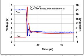
FIGURE 2-3: Internal Power Switch Short Response.
