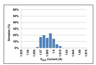
**FIGURE 2-17:** ILIM5 Trip Current Distribution<sup>(1)</sup>.
