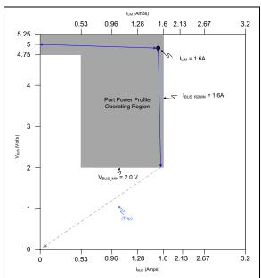
FIGURE 6-4: I<sub>LIM</sub> < I<sub>BUS R2MIN</sub> Example.
