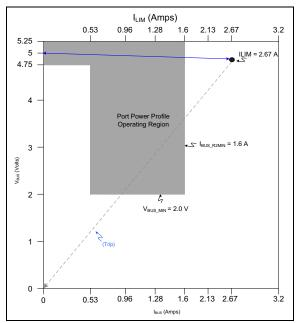
**FIGURE 6-5:**  $I_{LIM} > I_{BUS R2MIN}$  Example.
