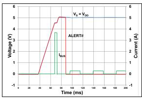
FIGURE 2-2: Power-Up Into a Short.
