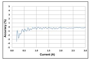
**FIGURE 2-10:** I<sub>BUS</sub> Measurement Accuracy.
