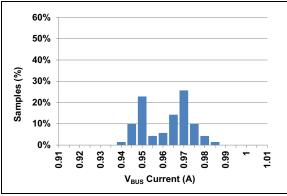
**FIGURE 2-14:** ILIM2 Trip Current Distribution<sup>(1)</sup>.
