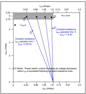
FIGURE 6-3: Current Limiting in CC Mode.
