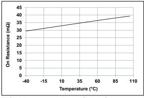
**FIGURE 2-5:** Power Switch On Resistance vs. Temperature.
