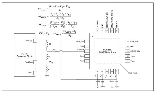
FIGURE 5-3: Boost# Pin Usage.
