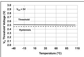
**FIGURE 2-8:** V<sub>S</sub> Undervoltage Threshold vs. Temperature.
