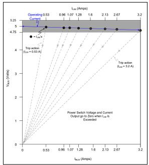
FIGURE 6-1: Current Limiting in Trip Mode.
