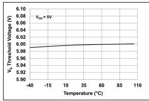
**FIGURE 2-7:**  $V_S$  Overvoltage Threshold vs. Temperature.
