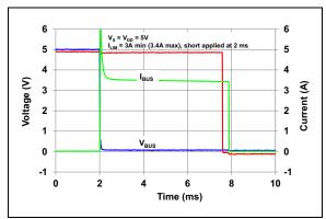
**FIGURE 2-1:** Short Applied After Power-Up.
