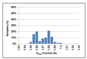
**FIGURE 2-16:** ILIM4 Trip Current Distribution<sup>(1)</sup>.
