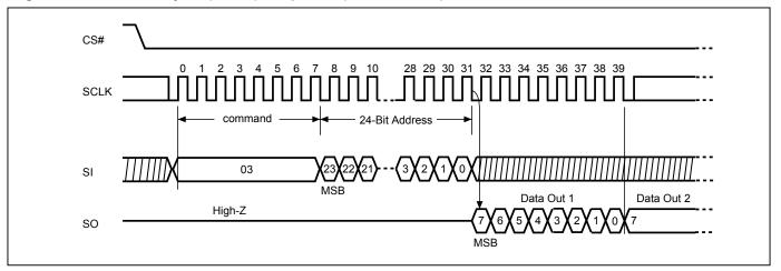
Figure 15. Read at Higher Speed (FAST\_READ) Sequence (Command 0B)
