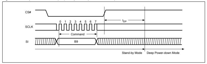
Figure 25. RDP and Read Electronic Signature (RES) Sequence (Command AB)
