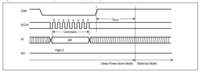
Figure 27. Read Electronic Manufacturer & Device ID (REMS) Sequence (Command 90 or EF or DF)
