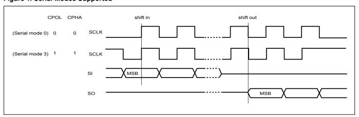
Figure 1. Serial Modes Supported
