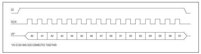
Figure 11. 3-Wire Single-Byte Transfer
