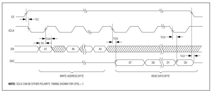
Figure 3. Timing Diagram: SPI Read Data Transfer
