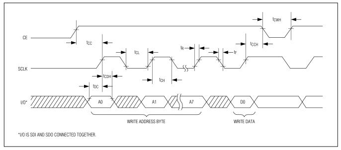
Figure 2. Timing Diagram: 3-Wire Write Data Transfer
