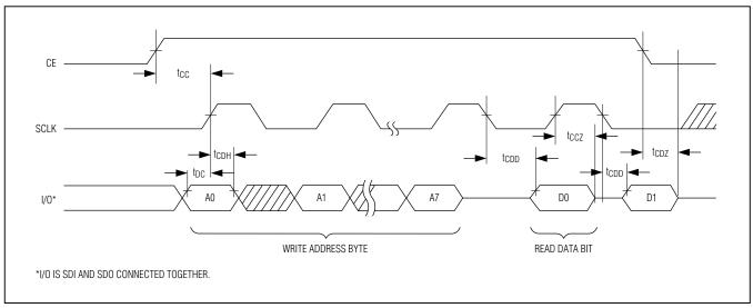
Figure 1. Timing Diagram: 3-Wire Read Data Transfer
