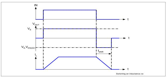
Figure 7 Switching an inductance
