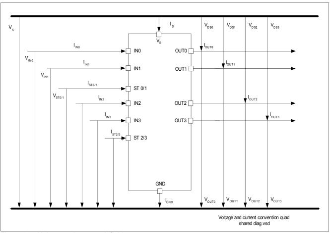
Figure 3 Voltage and current definition
