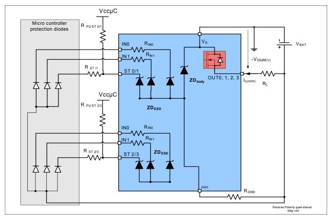
Figure 10 Reverse polarity protection with external components
