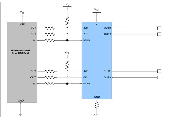
Figure 17 Application diagram with BTS4130QGA
