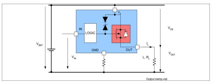
Figure 6 Output clamp (OUT0 and OUT1)
