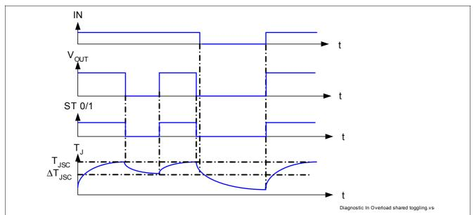
Figure 15 Sense signal in overtemperature condition
