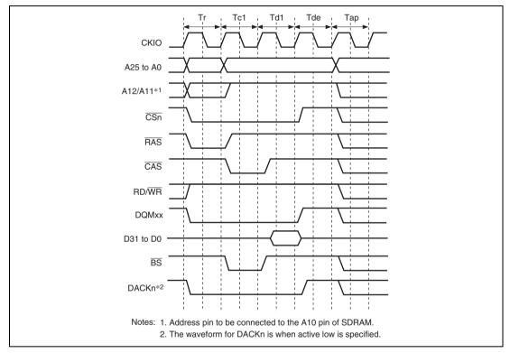
Figure 9.16 Basic Timing for Single Read (Auto-Precharge)
