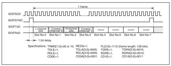
Figure 21.19 Transmit and Receive Timing (16-Bit Stereo Data (4))
