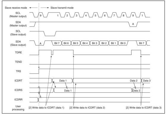
Figure 20.9 Slave Transmit Mode Operation Timing (1)
