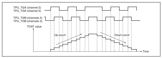
Figure 15.15 Example of Phase Counting Mode 1 Operation
