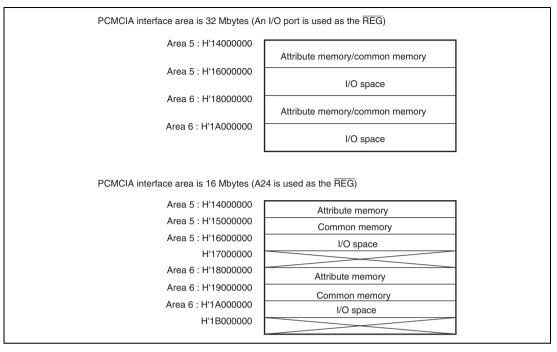
Figure 9.40 Example of PCMCIA Space Assignment (CS5BWCR.SA[1:0] = B'10, CS6BWCR.SA[1:0] = B'10)
