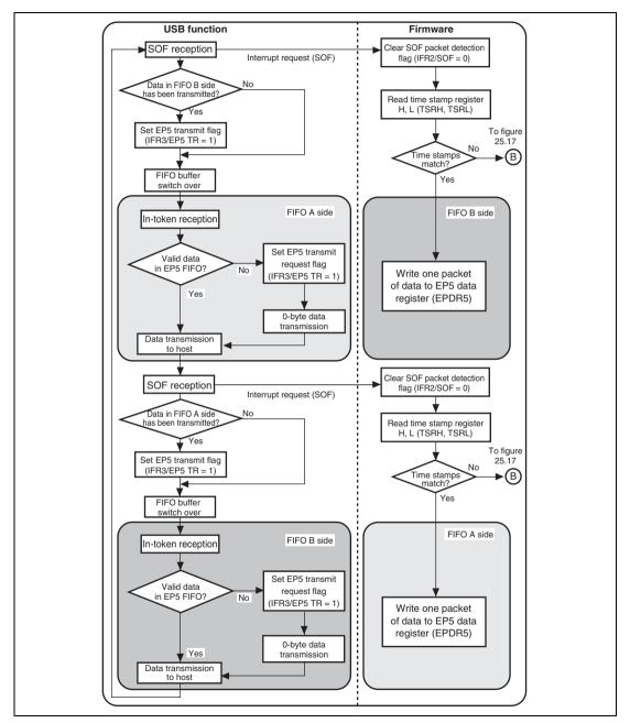
Figure 25.16 EP5 Isochronous-In Transfer Operation (SOF is Normal)
