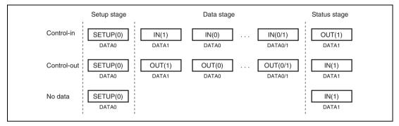
Figure 25.5 Transfer Stages in Control Transfer
