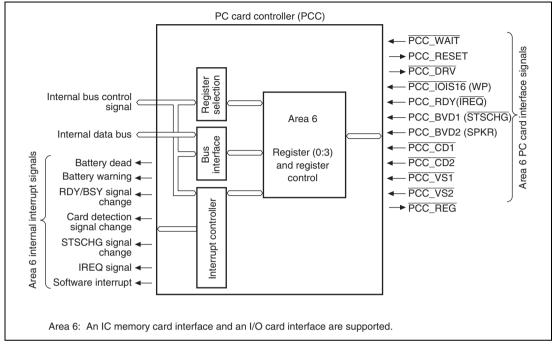
Figure 29.1 PC Card Controller Block Diagram
