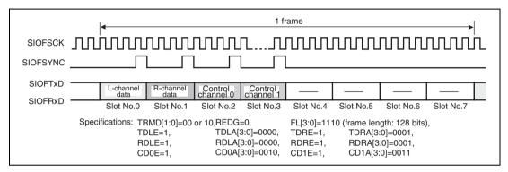
Figure 21.20 Transmit and Receive Timing (16-Bit Stereo Data)
