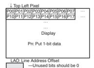
5. Packed 2bpp (Pixel Alignment in Byte is Little Endian)
