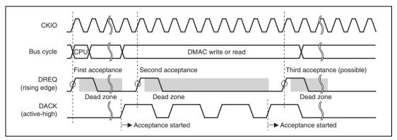
Figure 10.19 Timing of DREQ Input Detection by Edge Detection in Cycle Stealing Mode (DACK is Divided into Four due to Idle Cycle Insertion between Access Cycles and So DREQ Sampling is Accepted One Extra Time)
