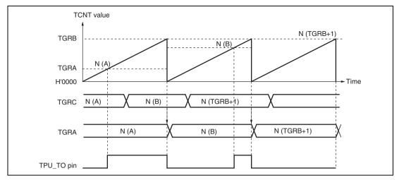
Figure 15.10 Example of Buffer Operation
