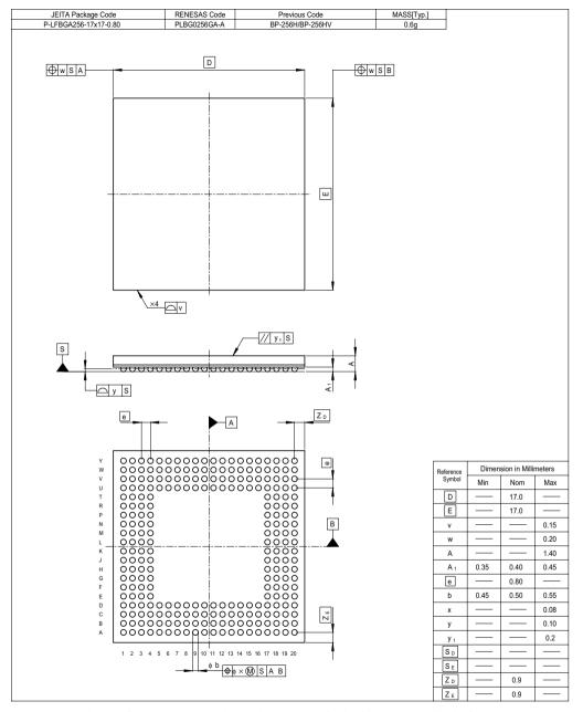
Figure C.1 Package Dimensions (PLBG0256GA-A (BP-256H/HV))
