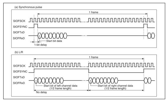
Figure 21.3 Serial Data Synchronization Timing
