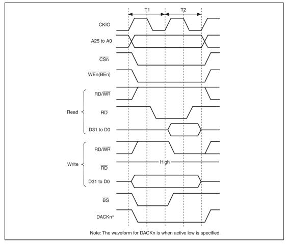
Figure 9.33 Basic Access Timing for Byte-Selection SRAM (BAS = 1)
