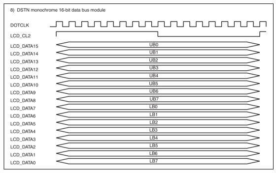
Figure 26.17 Clock and LCD Data Signal Example (DSTN Monochrome 16-Bit Data Bus Module)
