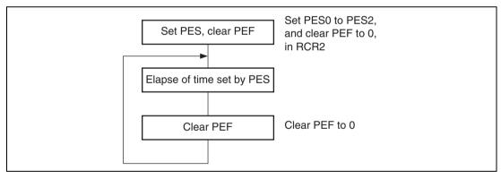
Figure 17.5 Using Periodic Interrupt Function
