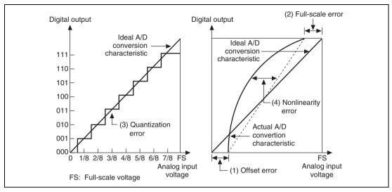
Figure 27.7 Definitions of A/D Conversion Accuracy
