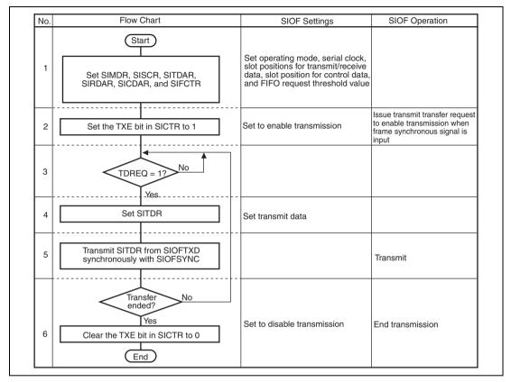
Figure 21.11 Example of Transmit Operation in Slave Mode
