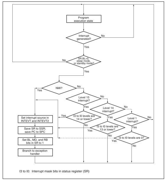
Figure 8.3 Interrupt Operation Flowchart
