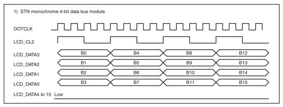
Figure 26.10 Clock and LCD Data Signal Example
