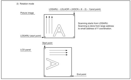
Figure 26.9 Operation for Hardware Rotation (Rotation Mode)
