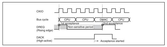
Figure 10.13 Example of DREQ Input Detection in Cycle Steal Mode Edge Detection
