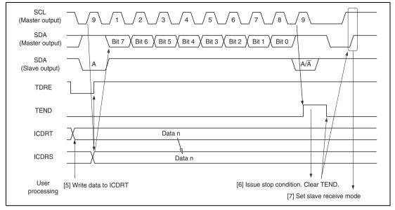
Figure 20.6 Master Transmit Mode Operation Timing (2)
