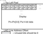
4. Packed 1bpp (Pixel Alignment in Byte is Little Endian)
