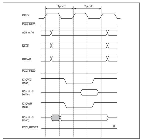
Figure 29.7 PCMCIA I/O Card Interface Basic Timing
