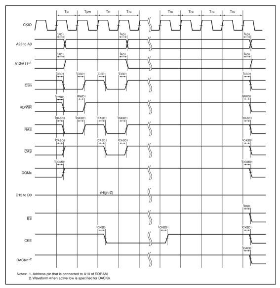
Figure 38.35 Self Refresh Timing of SDRAM (TRP = 2 Cycles)
