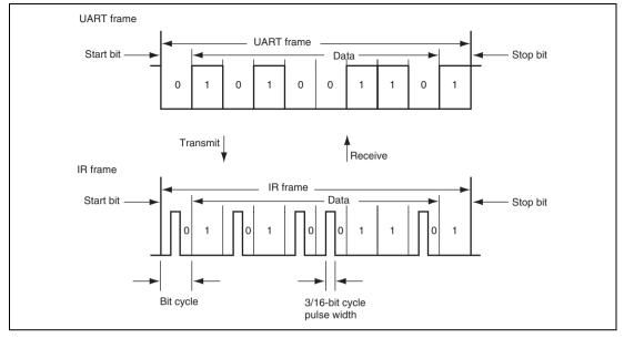
Figure 19.2 Transmit/Receive Operation
