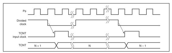
Figure 14.4 Count Timing when Internal Clock is Operating
