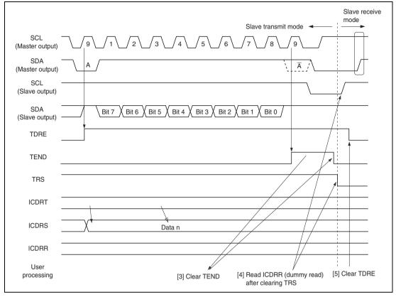
Figure 20.10 Slave Transmit Mode Operation Timing (2)
