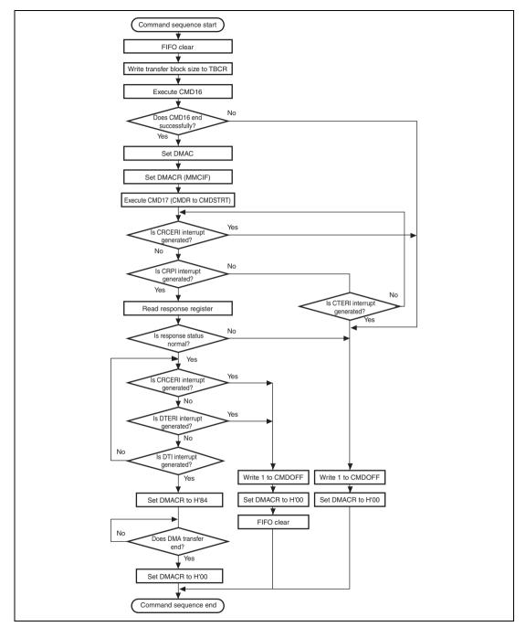
Figure 31.23 Operational Flowchart for Read Sequence (Single Block Transfer)
