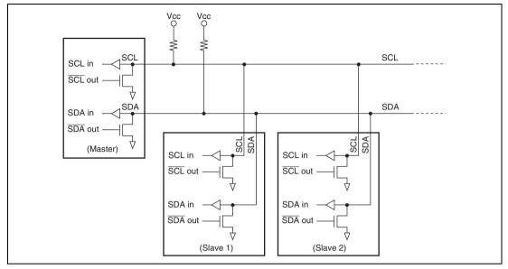
Figure 20.2 External Circuit Connections of I/O Pins
