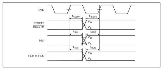
Figure 38.9 Interrupt Signal Input Timing
