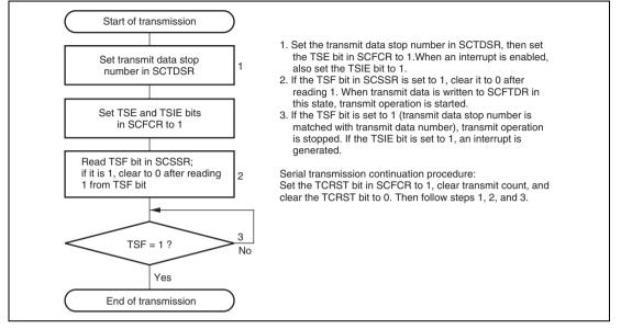
Figure 18.6 Transmit Data Stop Function Flowchart
