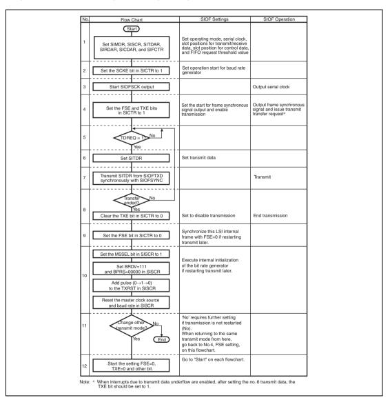
Figure 21.9 Example of Transmit Operation in Master Mode
