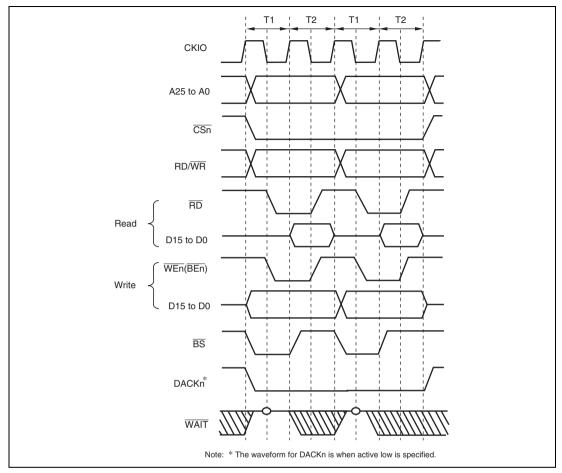
Figure 9.5 Continuous Access for Normal Space 2, Bus Width = 16 bits, Longword Access, CSnWCR.WM Bit = 1 (Access Wait = 0, Cycle Wait = 0)
