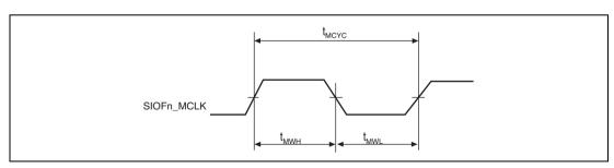
Figure 38.53 SIOF\_MCLK Input Timing
