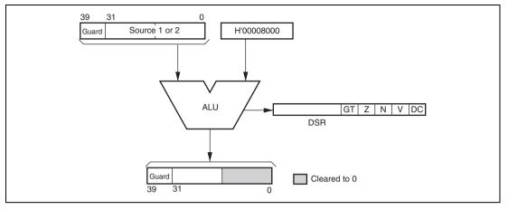
Figure 3.20 Rounding Operation Flow
