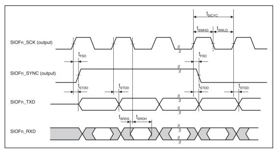
Figure 38.56 SIOF Transmission/Reception Timing (Master Mode 2, Fall Sampling)
