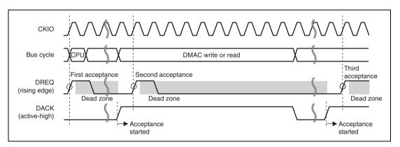
Figure 10.20 Timing of DREQ Input Detection by Edge Detection in Cycle Stealing Mode (DACK is Not Divided By Idle Cycle Insertion between Access Cycles and So DREQ Sampling is Accepted Normally)
