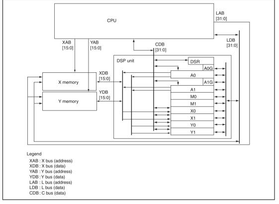
Figure 3.4 DSP Registers and Bus Connections
