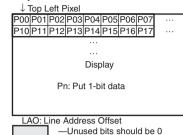
2. Packed 2bpp (Pixel Alignment in Byte is Big Endian) [Windows CE Recommended Format]
