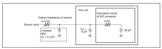
Figure 27.8 Analog Input Circuit Example
