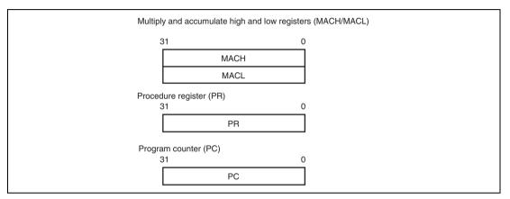
Figure 2.5 System Registers and Program Counter
