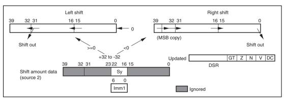
Figure 3.17 Arithmetic Shift Operation Flow
