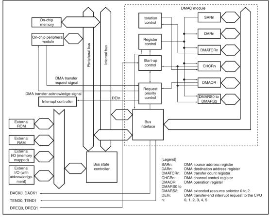
Figure 10.1 Block Diagram of DMAC
