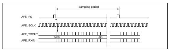
Figure 22.5 AFE Serial Interface
