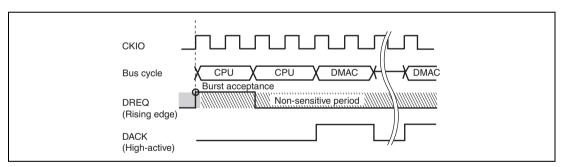
Figure 10.15 Example of DREQ Input Detection in Burst Mode Edge Detection
