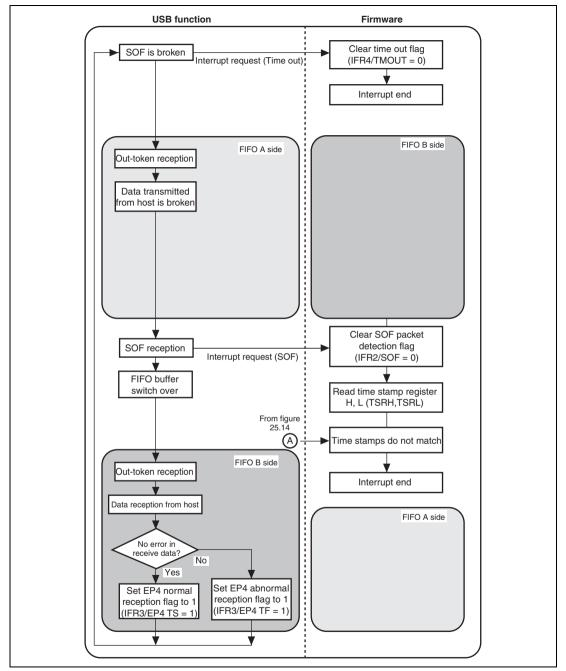
Figure 25.15 EP4 Isochronous-Out Transfer Operation (SOF is Broken)
