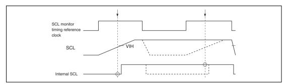
Figure 20.18 The Timing of the Bit Synchronous Circuit
