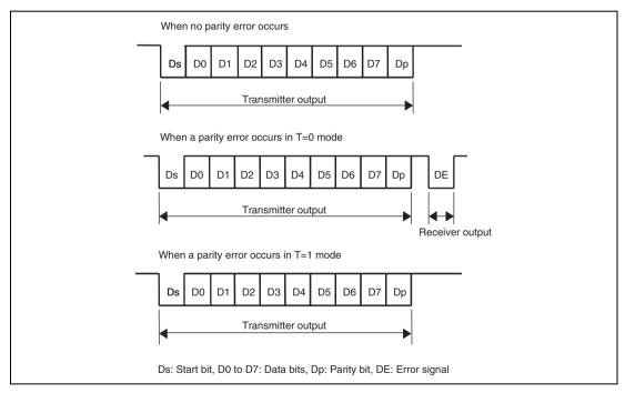
Figure 30.2 Data Format Used by Smart Card Interface
