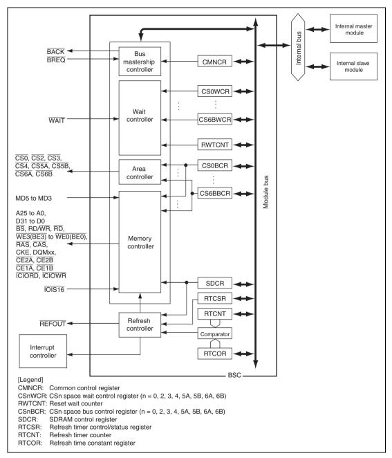
Figure 9.1 Block Diagram of BSC
