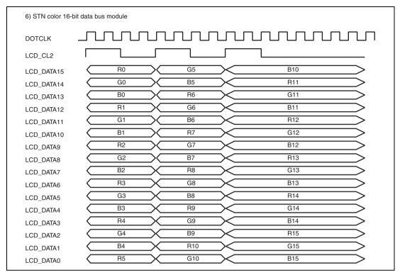
Figure 26.15 Clock and LCD Data Signal Example (STN Color 16-Bit Data Bus Module)
