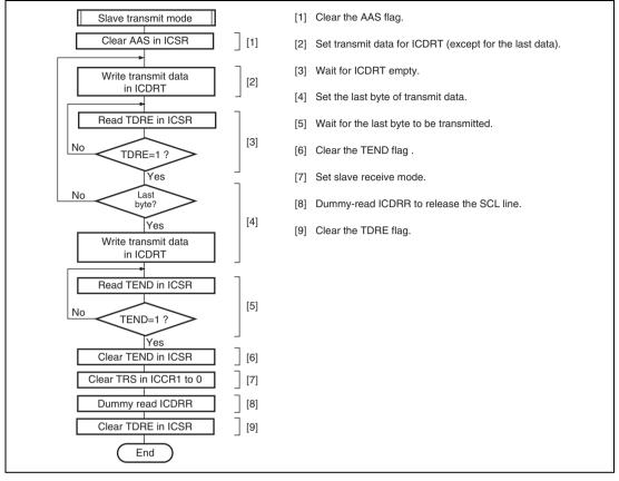
Figure 20.16 Sample Flowchart for Slave Transmit Mode
