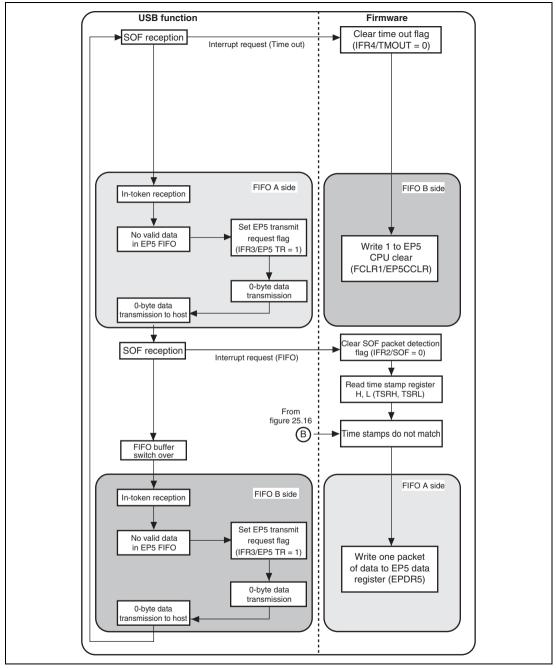
Figure 25.17 EP5 Isochronous-In Transfer Operation (SOF in Broken)
