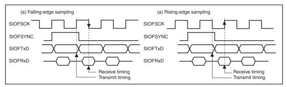
Figure 21.4 SIOF Transmit/Receive Timing
