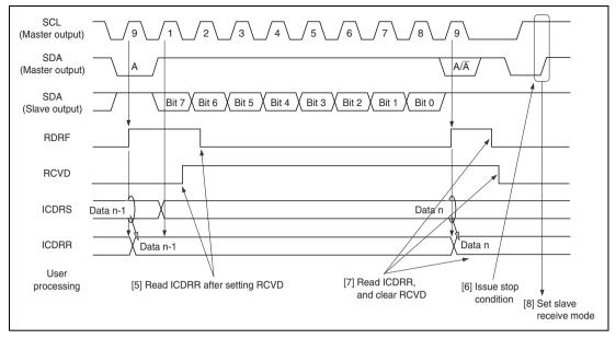
Figure 20.8 Master Receive Mode Operation Timing (2)
