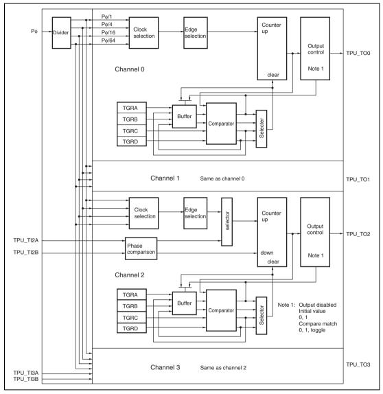
Figure 15.1 Block Diagram of TPU
