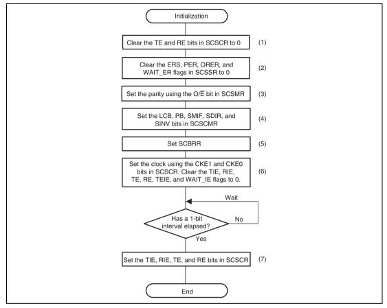
Figure 30.4 Example of Initialization Flow
