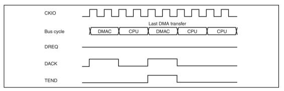
Figure 10.17 Example of DMA Transfer End in Cycle Steal Mode Level Detection
