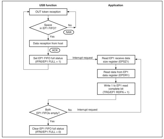
Figure 25.11 EP1 Bulk-Out Transfer Operation
