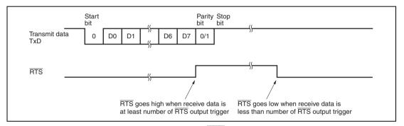
Figure 18.11 Example of  $\overline{RTS}$  Control Operation
