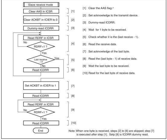
Figure 20.17 Sample Flowchart for Slave Receive Mode
