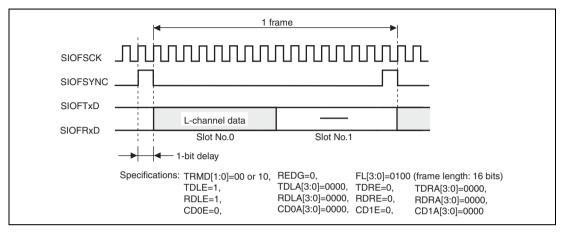
Figure 21.14 Transmit and Receive Timing (8-Bit Monaural Data (2))
