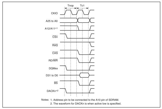
Figure 9.23 Single Write Timing (Bank Active, Same Row Address)
