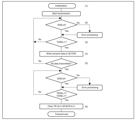
Figure 30.5 Example of Transmit Processing
