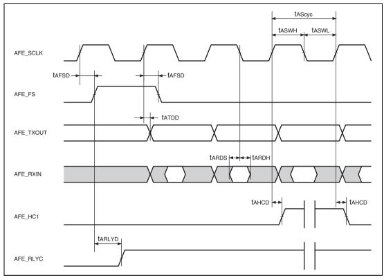
Figure 38.59 AFEIF Module AC Timing
