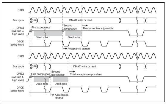
Figure 10.21 Timing of DREQ Input Detection by Level Detection in Cycle Stealing Mode (DACK is Divided into Four due to Idle Cycle Insertion between Access Cycles and So **DREQ Sampling is Accepted One Extra Time)**
