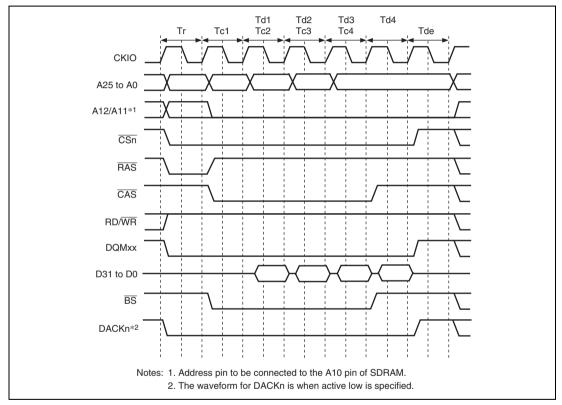
Figure 9.19 Burst Read Timing (No Auto-Precharge)
