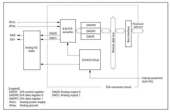
Figure 28.1 Block Diagram of D/A Converter
