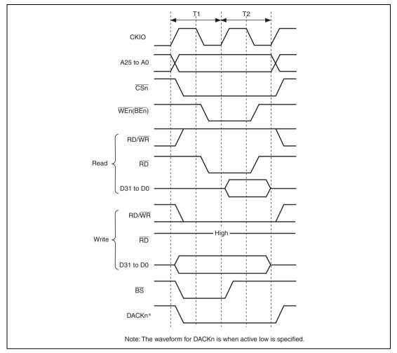
Figure 9.32 Basic Access Timing for Byte-Selection SRAM (BAS = 0)
