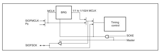
Figure 21.2 Serial Clock Supply
