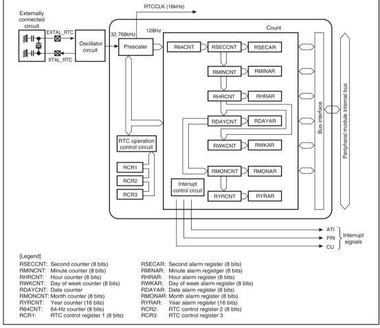
Figure 17.1 RTC Block Diagram
