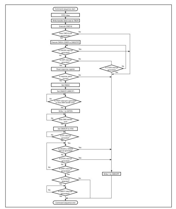
Figure 31.28 Operational Flowchart for Write Sequence (Single Block Transfer)
