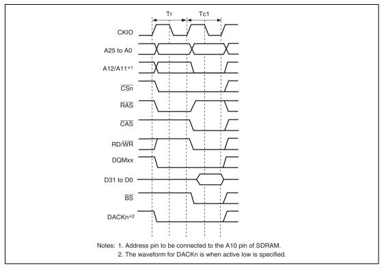
Figure 9.22 Single Write Timing (No Auto-Precharge)
