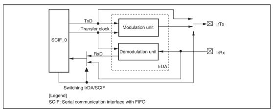
Figure 19.1 Block Diagram of IrDA
