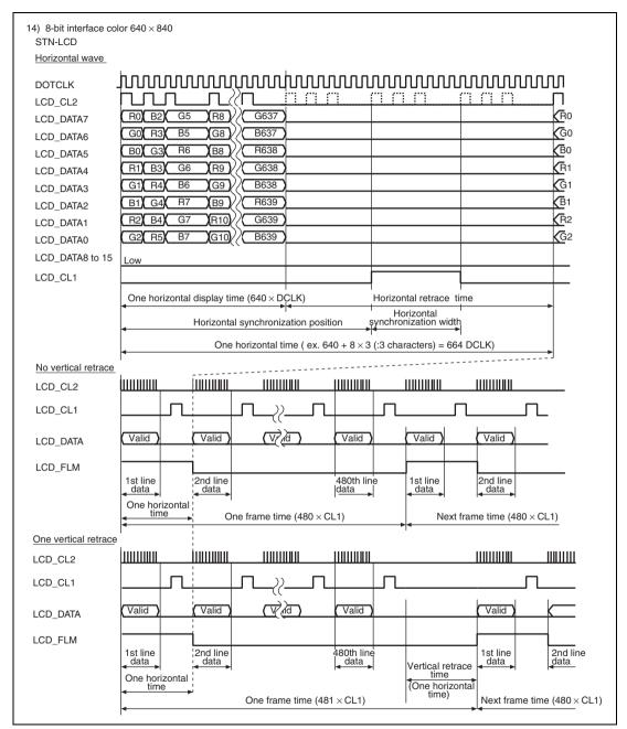
Figure 26.22 Clock and LCD Data Signal Example (8-Bit Interface Color 640 × 480)
