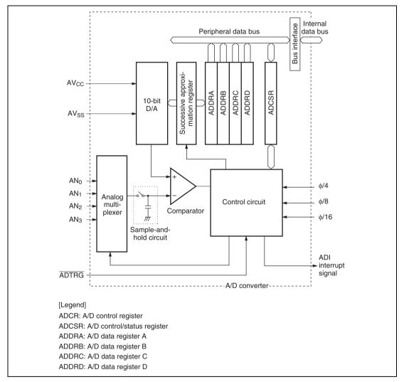
Figure 27.1 Block Diagram of A/D Converter
