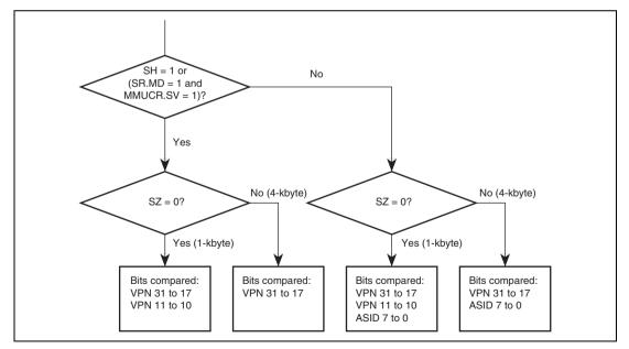
Figure 4.10 Objects of Address Comparison
