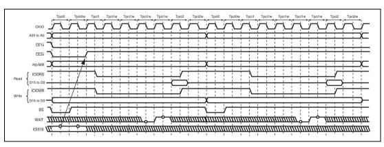
Figure 9.43 Timing for Dynamic Bus Sizing of PCMCIA I/O Card Interface (TED[3:0] = B'0010, TEH[3:0] = B'0001, Software Waits = 3)
