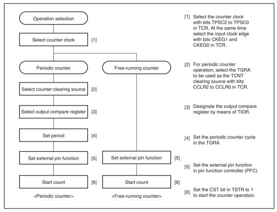
Figure 15.2 Example of Counter Operation Setting Procedure
