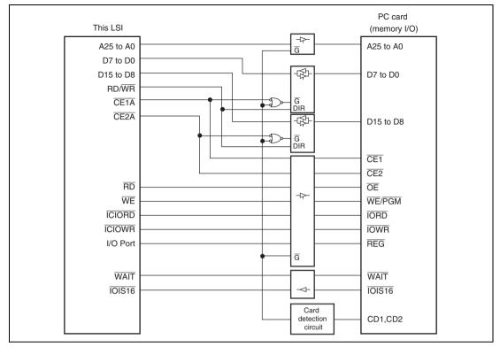
Figure 9.37 Example of PCMCIA Interface Connection
