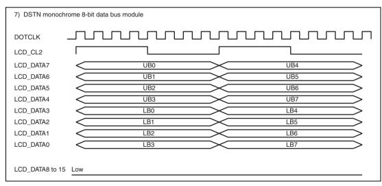
Figure 26.16 Clock and LCD Data Signal Example (DSTN Monochrome 8-Bit Data Bus Module)
