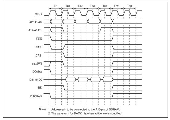
Figure 9.17 Basic Timing for Burst Write (Auto-Precharge)
