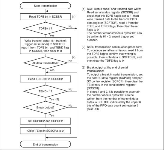
Figure 18.3 Sample Serial Transmission Flowchart
