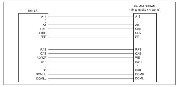
Figure 9.13 Example of 16-Bit Data-Width SDRAM Connection
