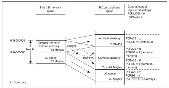
Figure 29.2 Continuous 32-Mbyte Area Mode
