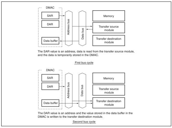
Figure 10.5 Data Flow of Dual Address Mode
