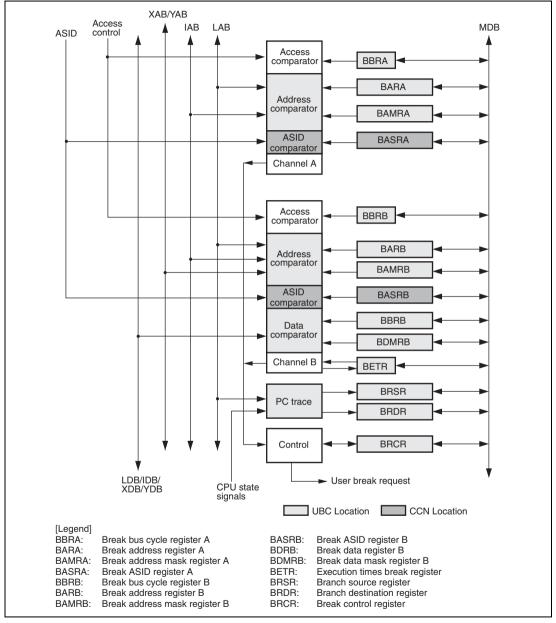
Figure 33.1 Block Diagram of UBC
