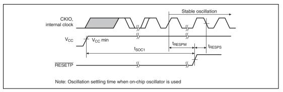
Figure 38.4 Power-On Oscillation Settling Time
