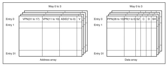
Figure 4.6 Overall Configuration of the TLB
