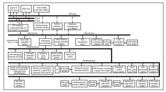
Figure 1.1 Block Diagram
