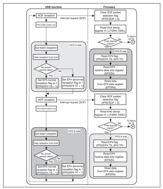
Figure 25.14 EP4 Isochronous-Out Transfer Operation (SOF is Normal)
