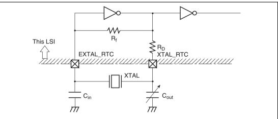
Notes: 1. Select either the C<sub>in</sub> or C<sub>out</sub> side for frequency adjustment variable capacitor according to requirements such as frequency range, degree of stability, etc.
