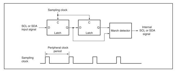
Figure 20.13 Block Diagram of Noise Conceller
