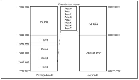
Figure 2.2 Virtual Address to External Memory Space Mapping
