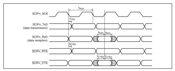
Figure 38.51 SCIF Input/Output Timing in Synchronous Mode
