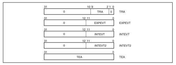
Figure 7.1 Register Bit Configuration
