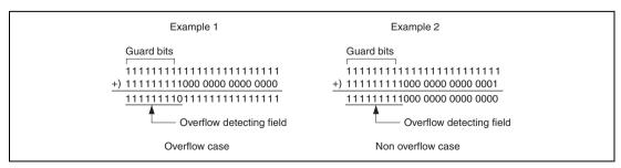
Figure 3.13 DC Bit Generation Examples in Overflow Mode
