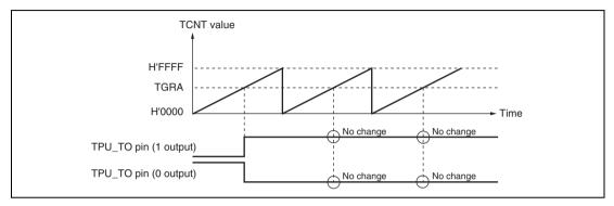
Figure 15.6 Example of 0 Output/1 Output Operation
