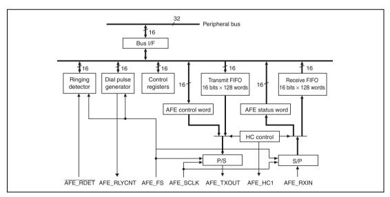
Figure 22.1 Block Diagram of AFE Interface
