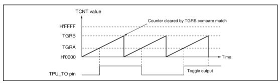
Figure 15.7 Example of Toggle Output Operation
