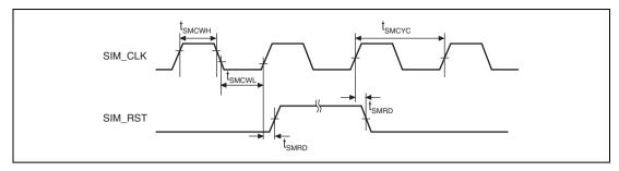
Figure 38.62 SIM Module Signal Timing
