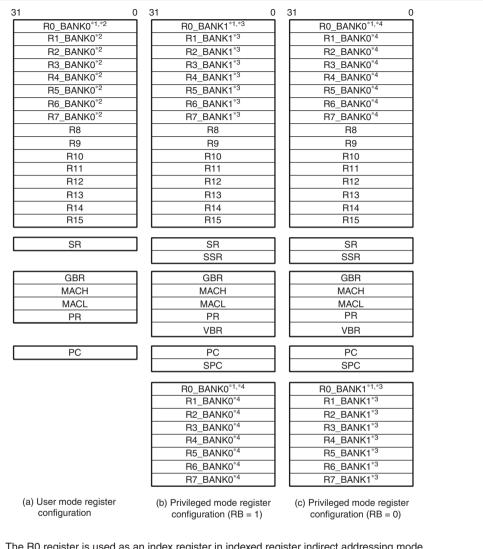
Notes: 1. The R0 register is used as an index register in indexed register indirect addressing mode and indexed GBR indirect addressing mode.
