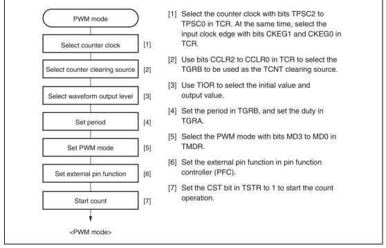
Figure 15.11 Example of PWM Mode Setting Procedure
