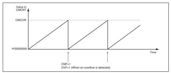
Figure 16.3 Counter Operation (Free-Running Operation)
