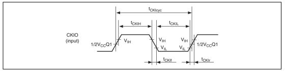
Figure 38.3 CKIO Clock Input Timing
