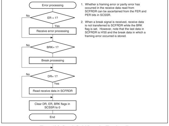
Figure 18.8 Sample Serial Reception Flowchart (2)
