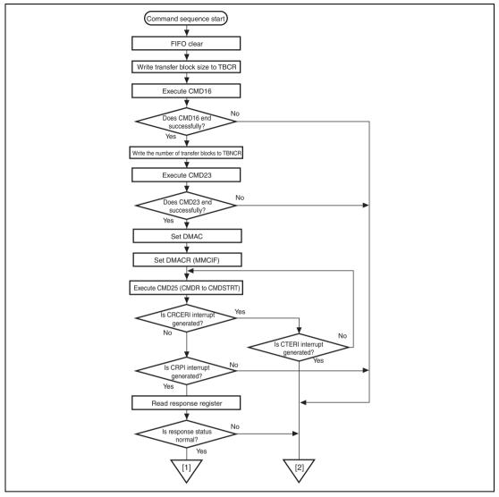
Figure 31.32 Operational Flowchart for Pre-defied Multiblock Write Transfer in Auto Mode (1)
