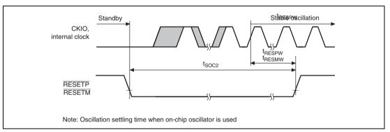
Figure 38.5 Oscillation Settling Time on Return from Standby (Return by Reset)
