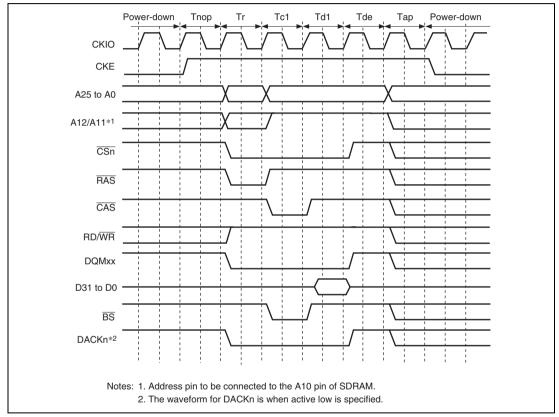
Figure 9.27 Access Timing in Power-Down Mode
