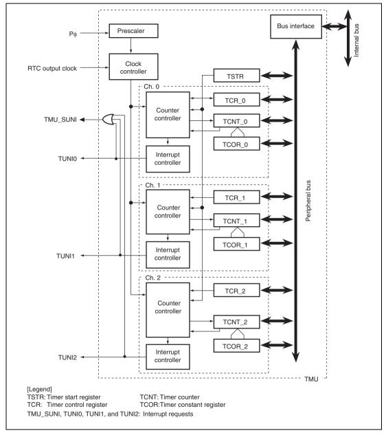
Figure 14.1 Block Diagram of TMU
