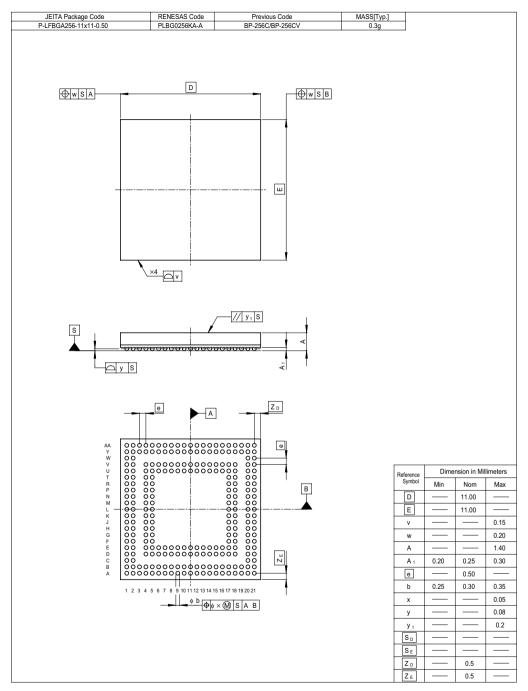
Figure C.2 Package Dimensions (PLBG0256KA-A (BP-256C/CV))
