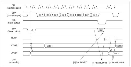
Figure 20.12 Slave Receive Mode Operation Timing (2)
