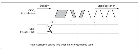
Figure 38.6 Oscillation Settling Time on Return from Standby (Return by NMI or IRQ)
