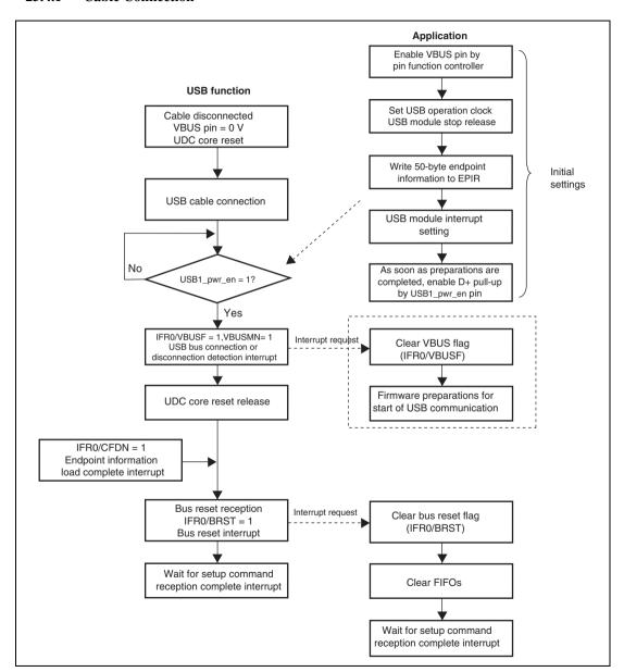
Figure 25.3 Cable Connection Operation
