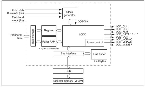
Figure 26.1 LCDC Block Diagram
