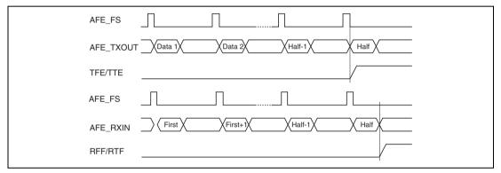
Figure 22.2 FIFO Interrupt Timing
