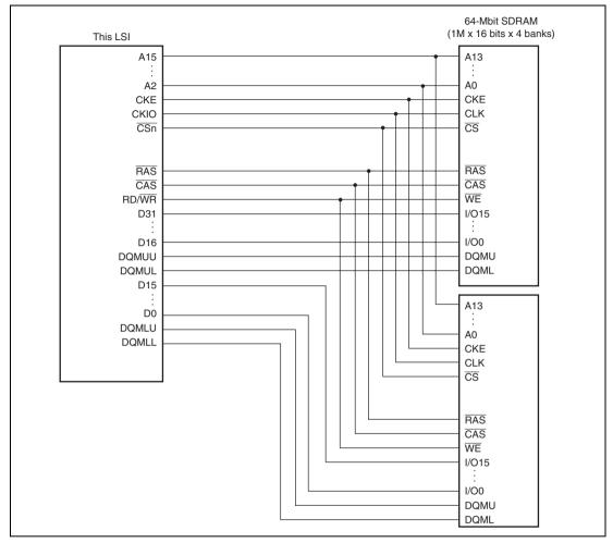
Figure 9.12 Example of 32-Bit Data-Width SDRAM Connection
