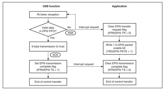
Figure 25.10 Status Stage (Control-Out) Operation
