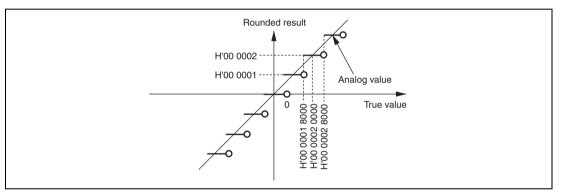
Figure 3.21 Definition of Rounding Operation
