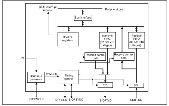
Figure 21.1 Block Diagram of SIOF
