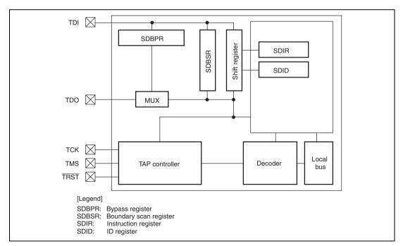
Figure 36.1 Block Diagram of H-UDI
