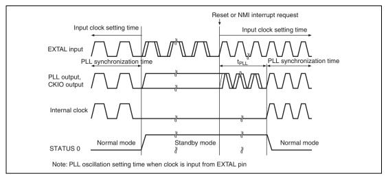
Figure 38.7 PLL Synchronization Settling Time by Reset, NMI or IRQ Interrupts
