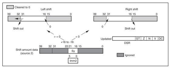
Figure 3.18 Logical Shift Operation Flow
