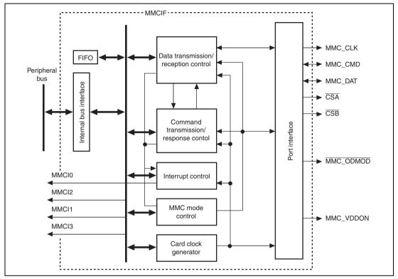
Figure 31.1 Block Diagram of MMCIF
