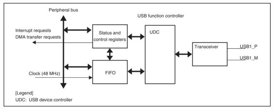
Figure 25.1 Block Diagram of USBF
