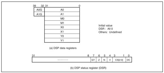
Figure 3.3 DSP Register Configuration
