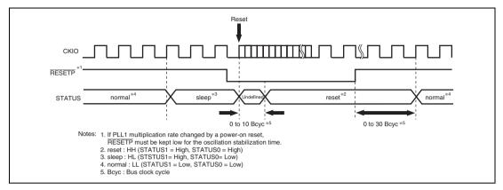
Figure 13.8 STATUS Output When Sleep Mode is Canceled by a Power-on Reset
