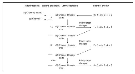
Figure 10.4 Changes in Channel Priority in Round-Robin Mode
