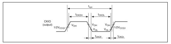
Figure 38.2 CKIO Clock Output Timing
