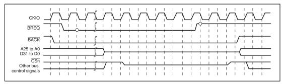
Figure 9.45 Bus Arbitration Timing
