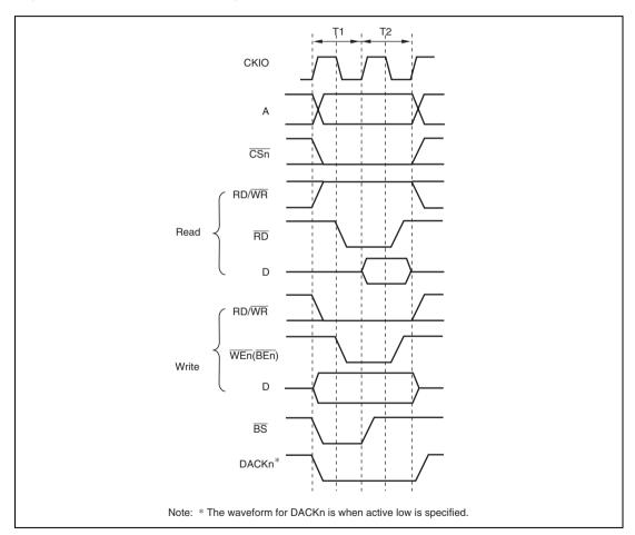
Figure 9.3 Normal Space Basic Access Timing (Access Wait 0)
