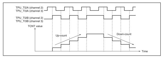
Figure 15.18 Example of Phase Counting Mode 4 Operation
