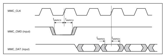
Figure 38.64 MMCIF Receive Timing (Rise Sampling)
