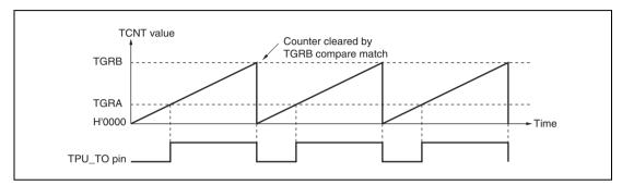
Figure 15.12 Example of PWM Mode Operation (1)
