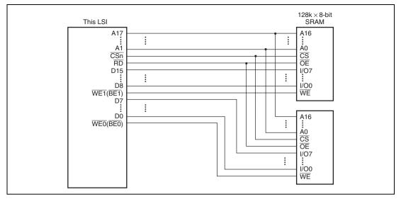
Figure 9.7 Example of 16-Bit Data-Width SRAM Connection
