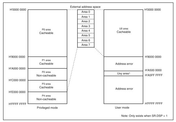
Figure 4.3 Virtual Address Space (MMUCR.AT = 0)
