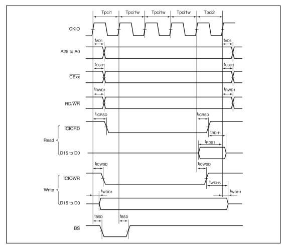
Figure 38.41 PCMCIA I/O Card Interface Bus Timing
