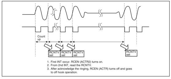
Figure 22.8 Ringing Detect Sequence
