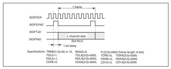
Figure 21.13 Transmit and Receive Timing (8-Bit Monaural Data (1))
