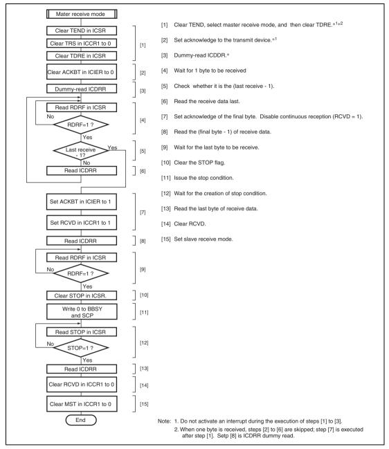
Figure 20.15 Sample Flowchart for Master Receive Mode
