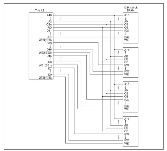
Figure 9.6 Example of 32-Bit Data-Width SRAM Connection
