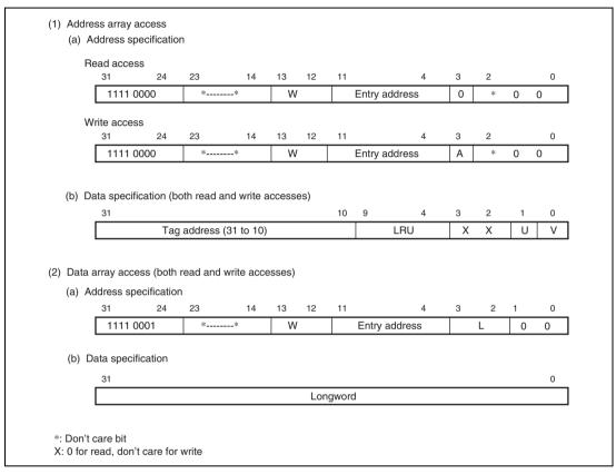
Figure 5.4 Specifying Address and Data for Memory-Mapped Cache Access (16-kbyte mode)
