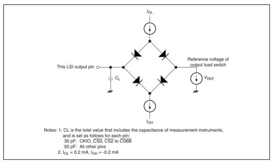
Figure 38.69 Output Load Circuit
