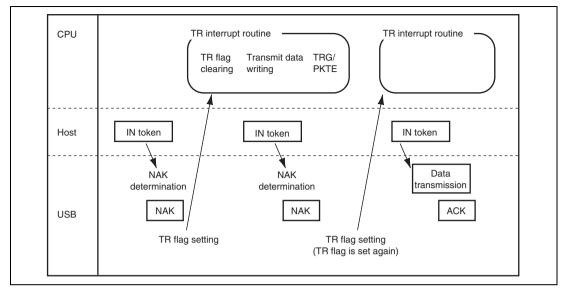
Figure 25.20 Set Timing of TR Interrupt Flag
