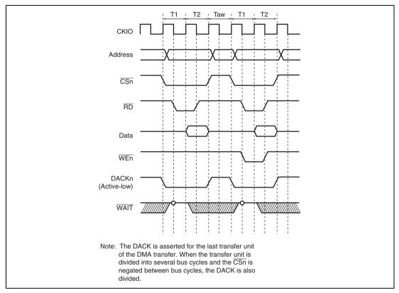
Figure 10.18 Example of BSC Ordinary Memory Access (No Wait, Idle Cycle 1, Longword Access to 16-Bit Device)
