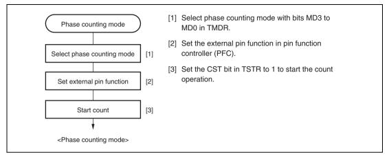
Figure 15.14 Example of Phase Counting Mode Setting Procedure
