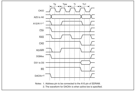
Figure 9.24 Single Write Timing (Bank Active, Different Row Addresses)
