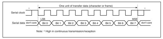
Figure 18.12 Data Format in Synchronous Communication
