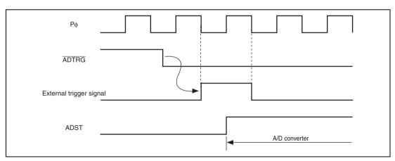
Figure 27.6 External Trigger Input Timing
