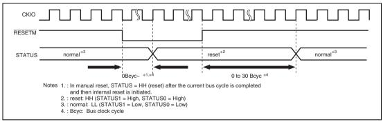
Figure 13.3 STATUS Output at Manual Reset
