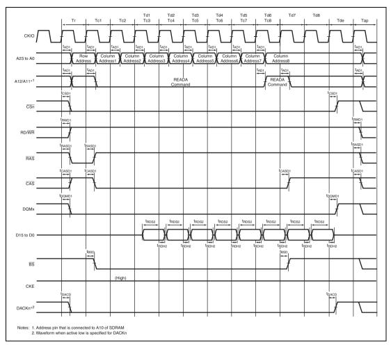
Figure 38.23 Burst Read Bus Cycle of SDRAM (Single Read × 8) (Auto Precharge Mode, CAS Latency 2, TRCD = 2 Cycles, TRP = 1 Cycle)
