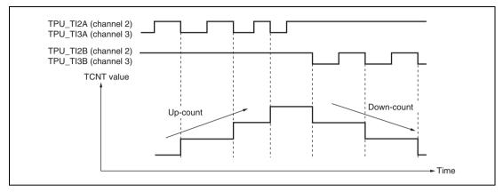
Figure 15.17 Example of Phase Counting Mode 3 Operation
