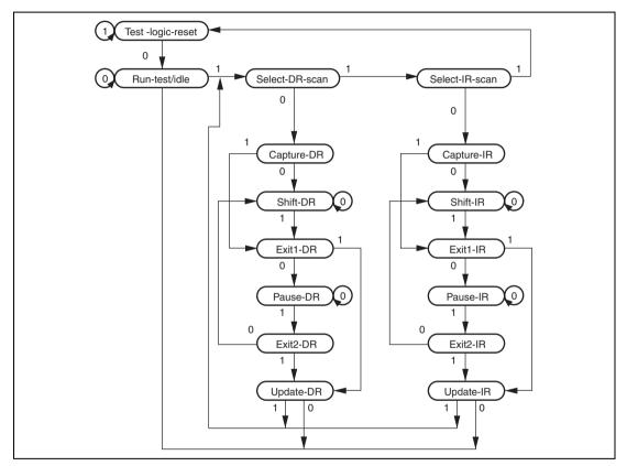
Figure 36.2 TAP Controller State Transitions
