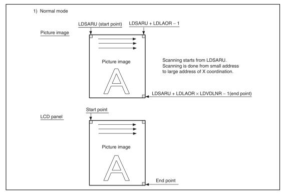
Figure 26.8 Operation for Hardware Rotation (Normal Mode)
