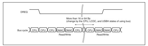
Figure 10.10 Example of DMA Transfer in Cycle Steal Intermittent Mode (Dual Address, DREQ Low Level Detection)
