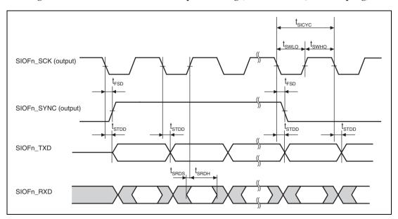
Figure 38.57 SIOF Transmission/Reception Timing (Master Mode 2, Rise Sampling)
