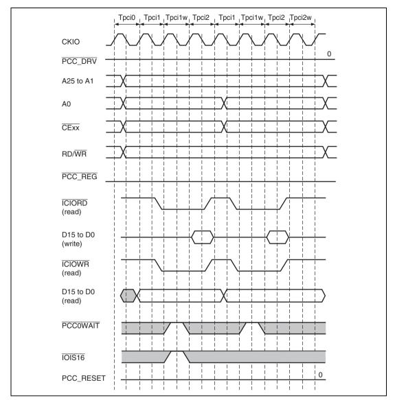
Figure 29.9 Dynamic Bus Sizing Timing for PCMCIA I/O Card Interface
