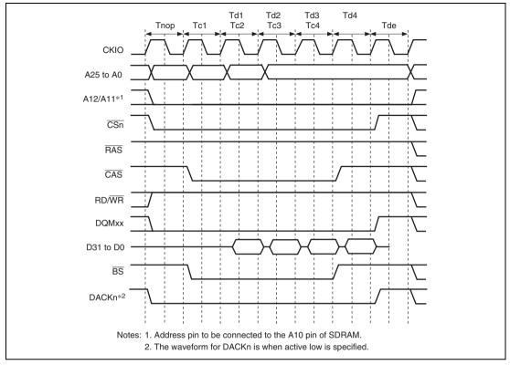
Figure 9.20 Burst Read Timing (Bank Active, Same Row Address)
