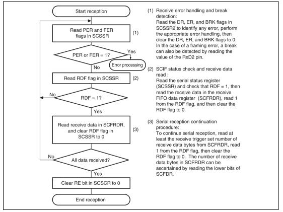
Figure 18.7 Sample Serial Reception Flowchart (1)
