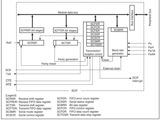
Figure 18.1 Block Diagram of SCIF
