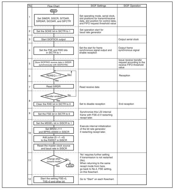
Figure 21.10 Example of Receive Operation in Master Mode
