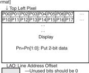
3. Packed 4bpp (Pixel Alignment in Byte is Big Endian) [Windows CE Recommended Format]
