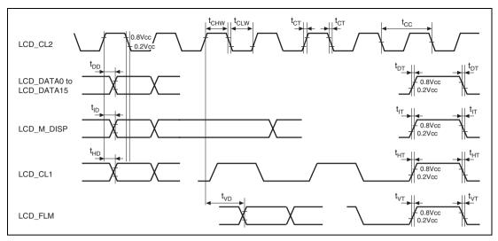
Figure 38.61 LCDC Module Signal Timing
