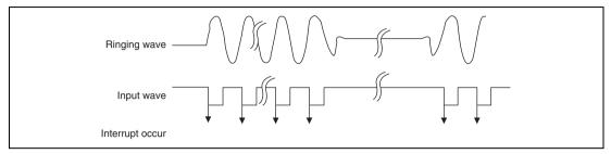
Figure 22.3 Ringing Interrupt Occurrence Timing
