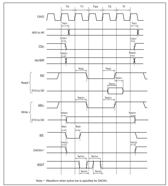
Figure 38.16 CS Extended Bus Cycle in Normal Space (SW = 1 Cycle, HW = 1 Cycle, External Wait 1 Input)
