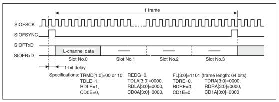
Figure 21.15 Transmit and Receive Timing (16-Bit Monaural Data (1))
