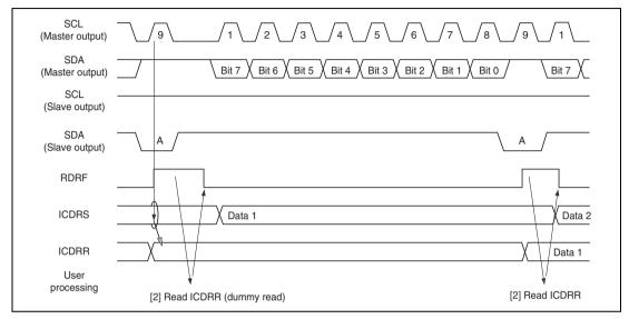
Figure 20.11 Slave Receive Mode Operation Timing (1)
