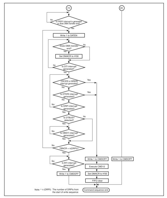
Figure 31.30 Operational Flowchart for Write Sequence (Pre-defined Multiblock Transfer) (2)
