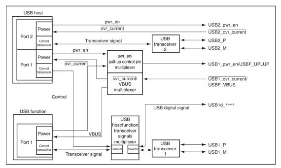
Figure 23.1 Block Diagram of USB PIN Multiplexer
