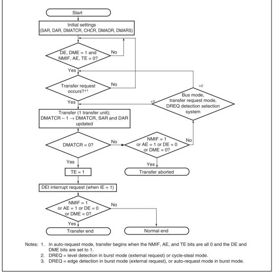
Figure 10.2 DMA Transfer Flowchart
