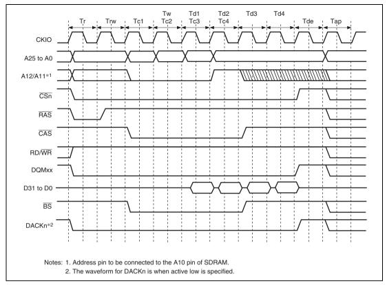
Figure 9.15 Burst Read Wait Specification Timing (Auto-Precharge)
