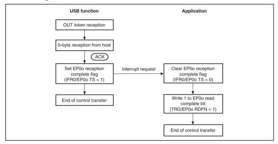
Figure 25.9 Status Stage (Control-In) Operation
