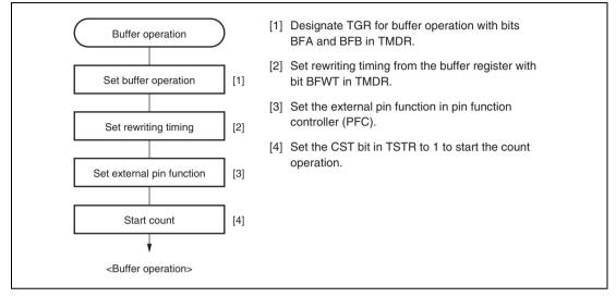
Figure 15.9 Example of Buffer Operation Setting Procedure
