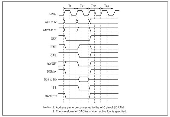
Figure 9.18 Basic Timing for Single Write (Auto-Precharge)
