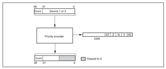
Figure 3.19 PDMSB Operation Flow
