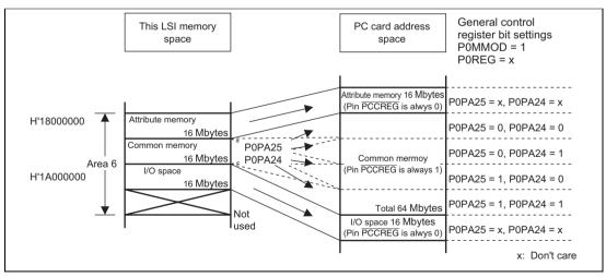
Figure 29.3 Continuous 16-Mbyte Area Mode (Area 6)
