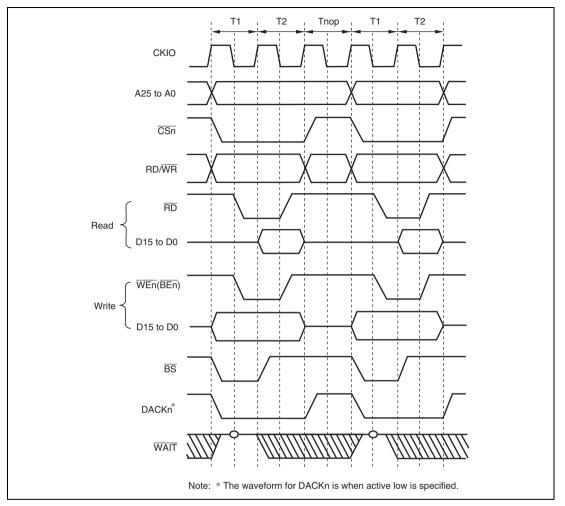
Figure 9.4 Continuous Access for Normal Space 1, Bus Width = 16 bits, Longword Access, **CSnWCR.WM** Bit = 0 (Access Wait = 0, Cycle Wait = 0)
