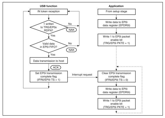
Figure 25.7 Data Stage (Control-In) Operation
