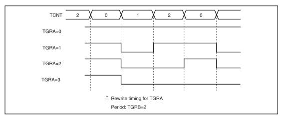
Figure 15.13 Examples of PWM Mode Operation (2)
