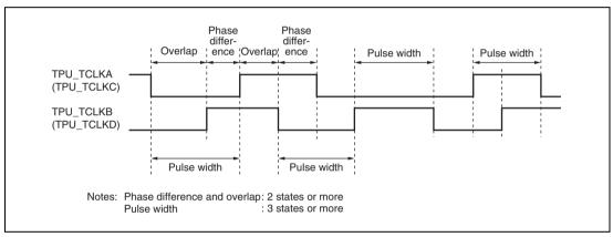
Figure 15.19 Phase Difference, Overlap, and Pulse Width in Phase Counting Mode
