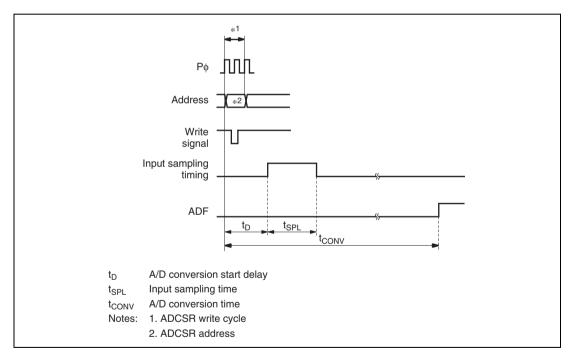
Figure 27.5 A/D Conversion Timing
