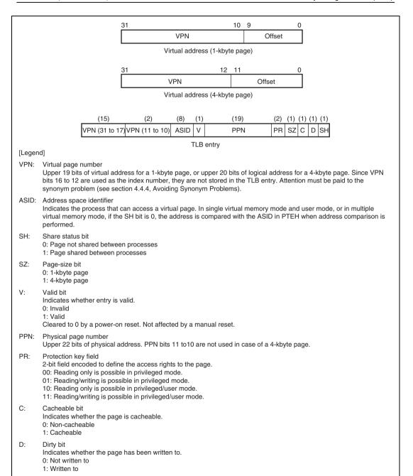
Figure 4.7 Virtual address and TLB Structure
