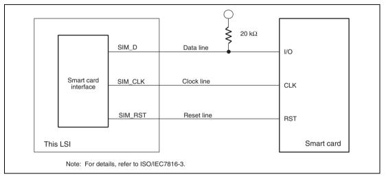
Figure 30.11 Example of Pin Connections in Smart Card Interface
