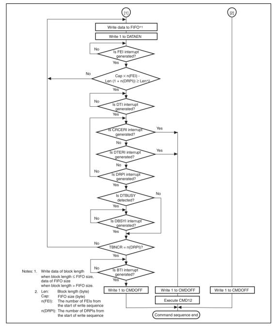
Figure 31.21 Operational Flowchart for Commands with Write Data (Pre-defined Multiblock Transfer) (2)
