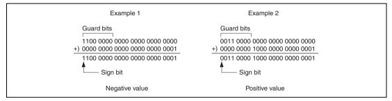
Figure 3.12 DC Bit Generation Examples in Negative Value Mode
