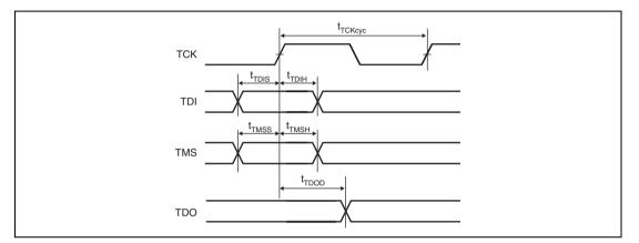
Figure 38.67 H-UDI Data Transfer Timing
