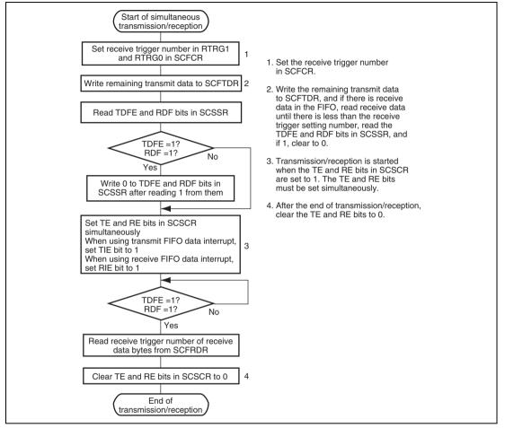
Figure 18.16 Sample Simultaneous Serial Transmission and Reception Flowchart (1)
