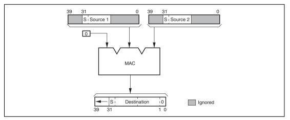
Figure 3.16 Fixed-Point Multiply Operation Flow
