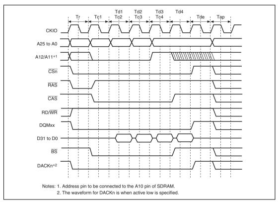
Figure 9.14 Burst Read Basic Timing (Auto-Precharge)
