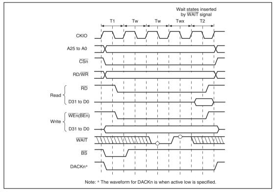
Figure 9.10 Wait State Timing for Normal Space Access (Wait State Insertion using WAIT Signal)
