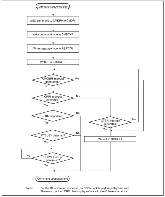
Figure 31.6 Operational Flowchart for Commands without Data Transfer
