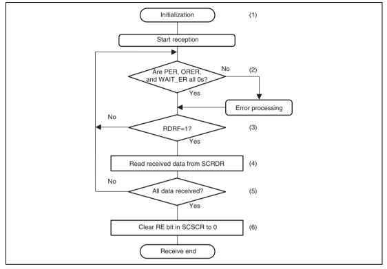
Figure 30.6 Example of Receive Processing
