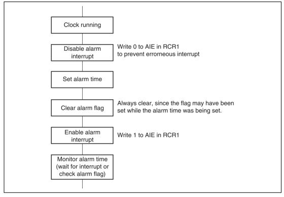
Figure 17.4 Using Alarm Function
