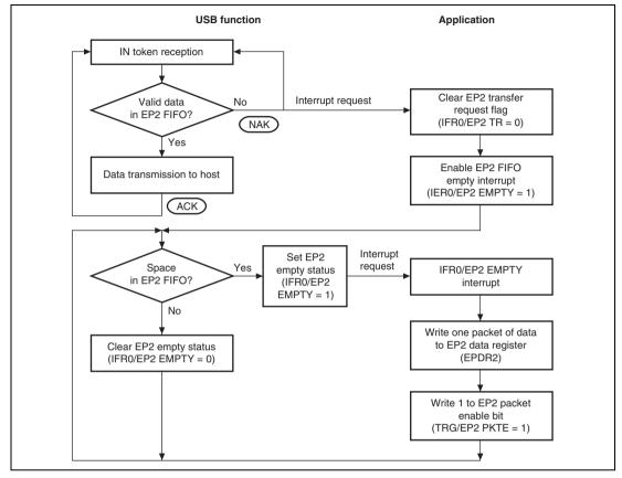
Figure 25.12 EP2 Bulk-In Transfer Operation
