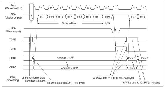
Figure 20.5 Master Transmit Mode Operation Timing (1)
