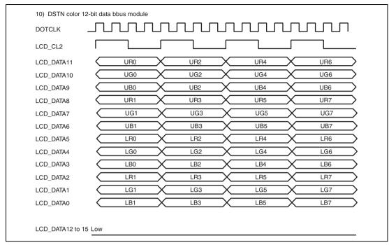
Figure 26.19 Clock and LCD Data Signal Example (DSTN Color 12-Bit Data Bus Module)
