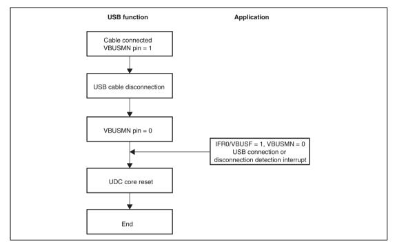
Figure 25.4 Cable Disconnection Operation
