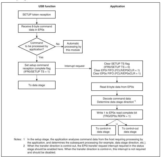
Figure 25.6 Setup Stage Operation
