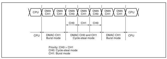
Figure 10.12 Bus State when Multiple Channels are Operating
