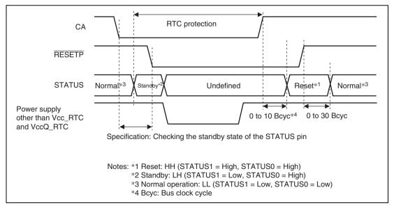
Figure 13.12 Timing When Power of Pins other than  $V_{\rm cc}$ -RTC and  $V_{\rm cc}Q$ -RTC is Off
