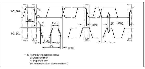
Figure 38.52 I<sup>2</sup>C Bus Interface Input/Output Timing
