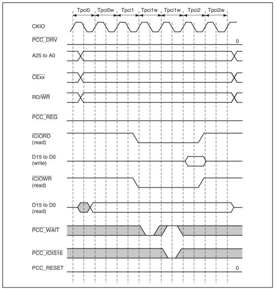
Figure 29.8 PCMCIA I/O Card Interface Wait Timing
