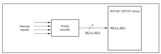
Figure 8.2 Example of IRL Interrupt Connection
