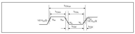
Figure 38.65 TCK Input Timing
