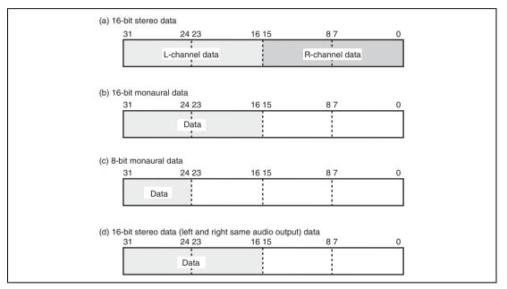
Figure 21.5 Transmit/Receive Data Bit Alignment
