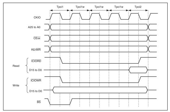
Figure 9.41 Basic Timing for PCMCIA I/O Card Interface
