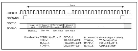
Figure 21.7 Control Data Interface (Slot Position)
