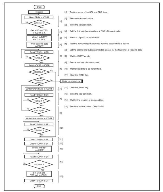
Figure 20.14 Sample Flowchart for Master Transmit Mode
