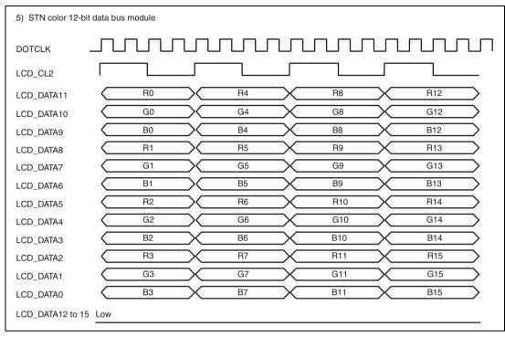
Figure 26.14 Clock and LCD Data Signal Example (STN Color 12-Bit Data Bus Module)
