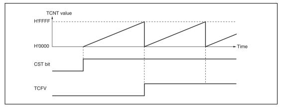
Figure 15.3 Free-Running Counter Operation
