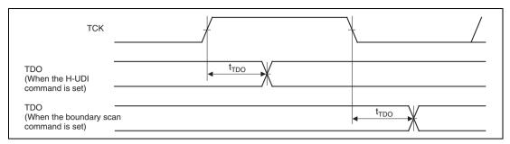
Figure 36.3 H-UDI Data Transfer Timing
