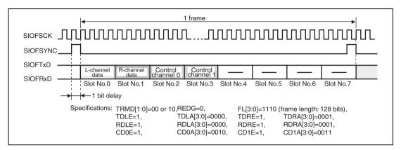
Figure 21.18 Transmit and Receive Timing (16-Bit Stereo Data (3))
