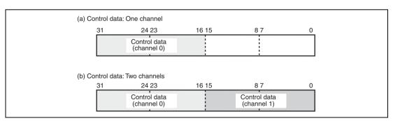
Figure 21.6 Control Data Bit Alignment
