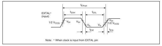
Figure 38.1 EXTAL Clock Input Timing
