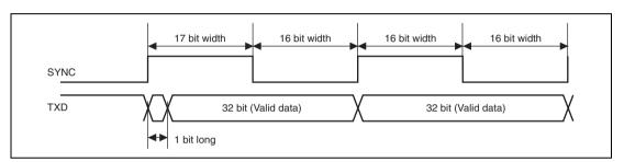
Figure 21.21 Frame Length (32-Bit)
