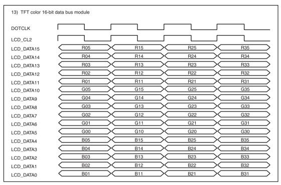
Figure 26.21 Clock and LCD Data Signal Example (TFT Color 16-Bit Data Bus Module)
