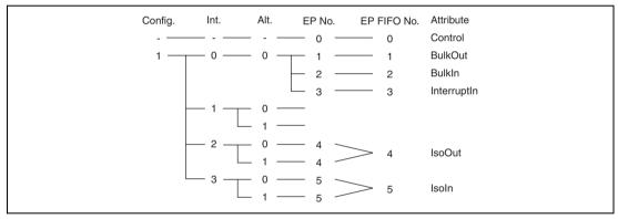
Figure 25.2 Example of Endpoint Configuration
