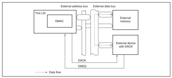
Figure 10.7 Data Flow in Single Address Mode
