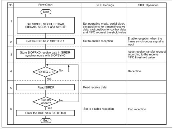
Figure 21.12 Example of Receive Operation in Slave Mode
