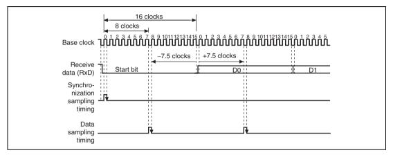
Figure 18.17 Receive Data Sampling Timing in Asynchronous Mode
