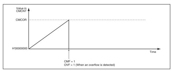
Figure 16.2 Counter Operation (One-Shot Operation)
