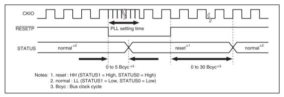
Figure 13.2 STATUS Output at Power-on Reset
