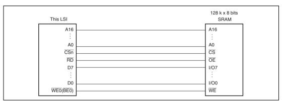
Figure 9.8 Example of 8-Bit Data-Width SRAM Connection
