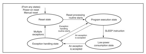
Figure 2.1 Processing State Transitions
