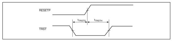
Figure 38.66 TRST Input Timing (Reset Hold)
