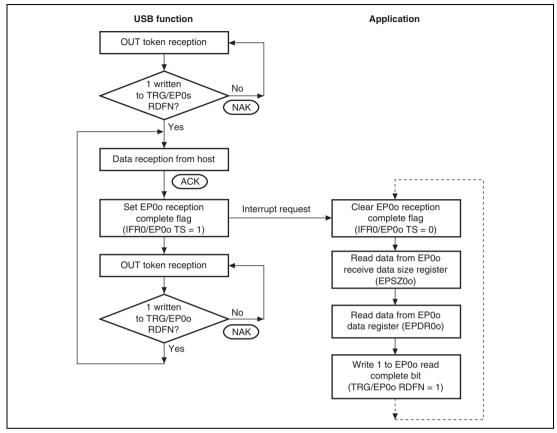
Figure 25.8 Data Stage (Control-Out) Operation
