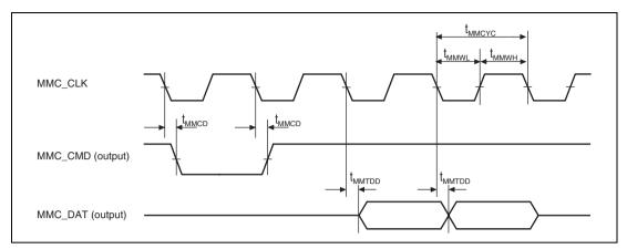
Figure 38.63 MMCIF Transmit Timing
