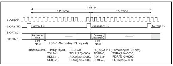
Figure 21.8 Control Data Interface (Secondary FS)
