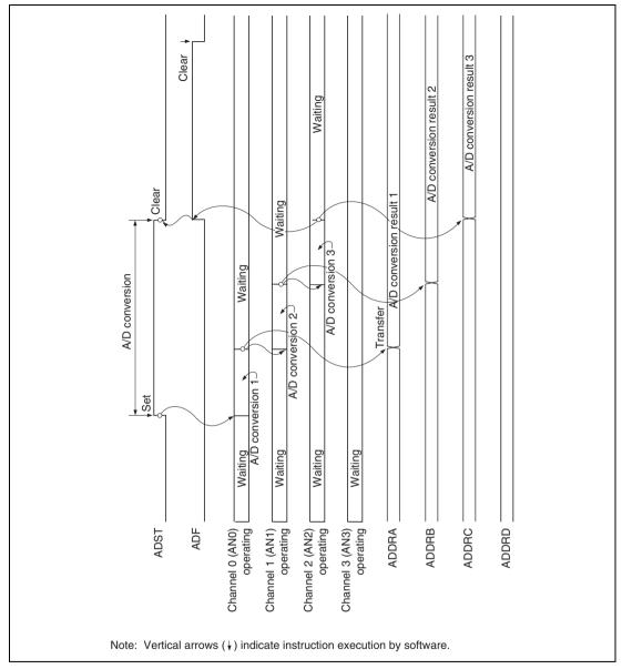
Figure 27.3 Example of A/D Converter Operation (Multi Mode, Channels AN0 to AN2 Selected)
