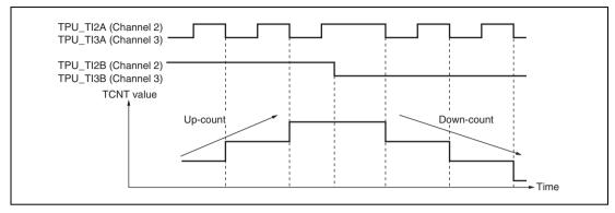
Figure 15.16 Example of Phase Counting Mode 2 Operation
