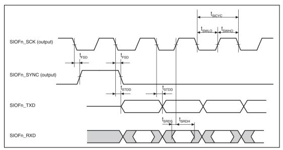
Figure 38.55 SIOF Transmission/Reception Timing (Master Mode 1, Rise Sampling)
