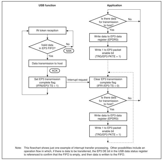
Figure 25.13 EP3 Interrupt-In Transfer Operation
