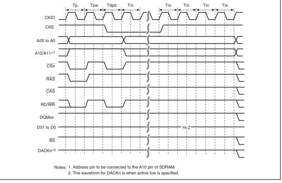
Figure 9.30 Transition Timing in Deep Power-Down Mode
