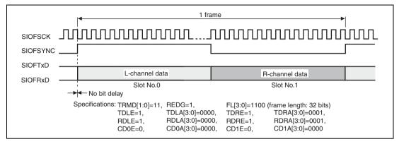
Figure 21.16 Transmit and Receive Timing (16-Bit Stereo Data (1))
