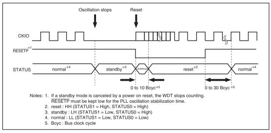
Figure 13.5 STATUS Output When Software Standby Mode is Canceled by a Power-on Reset
