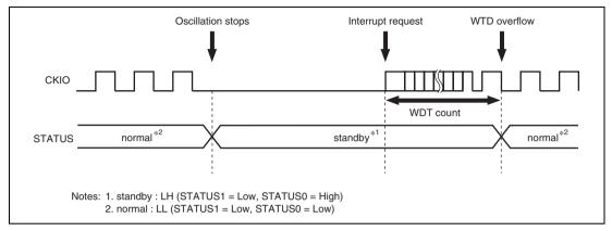
Figure 13.4 STATUS Output when Software Standby Mode is Canceled by an Interrupt
