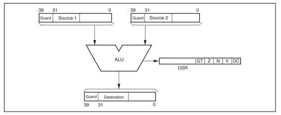
Figure 3.9 ALU Fixed-Point Arithmetic Operation Flow
