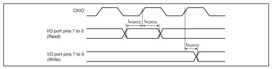
Figure 38.44 I/O Port Timing
