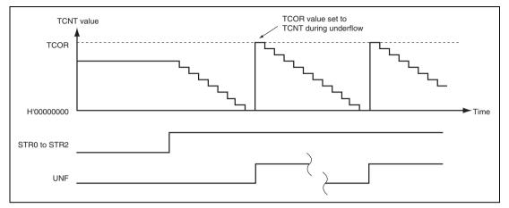
Figure 14.3 Auto-Reload Count Operation
