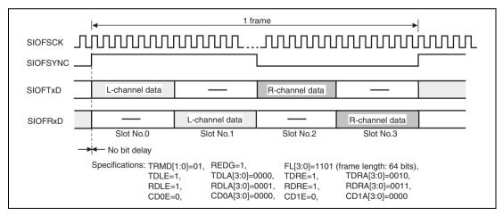
Figure 21.17 Transmit and Receive Timing (16-Bit Stereo Data (2))
