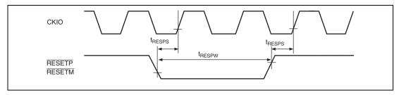
Figure 38.8 Reset Input Timing
