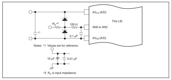
Figure 27.9 Example of Analog Input Protection Circuit
