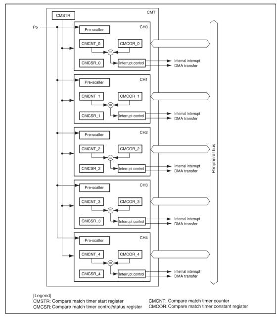
Figure 16.1 Block Diagram of CMT
