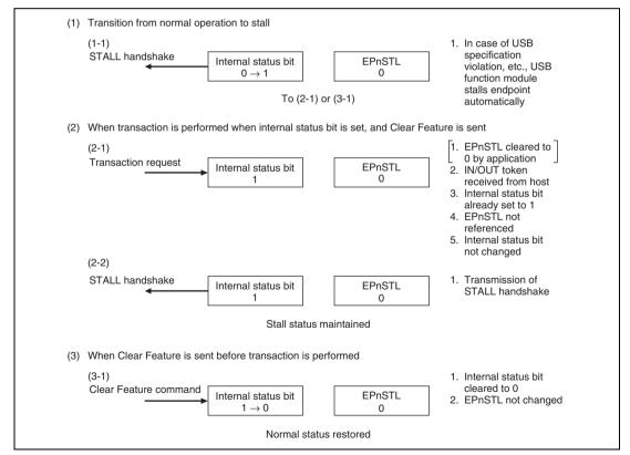
Figure 25.19 Automatic Stall by USB Function Controller
