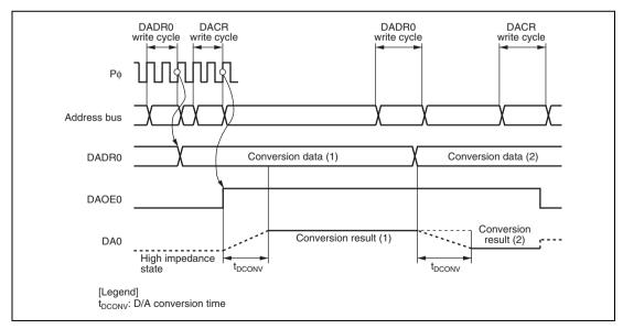
Figure 28.2 D/A Converter Operation Example
