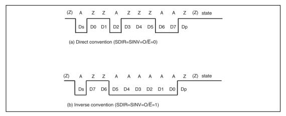
Figure 30.3 Examples of Start Character Waveforms
