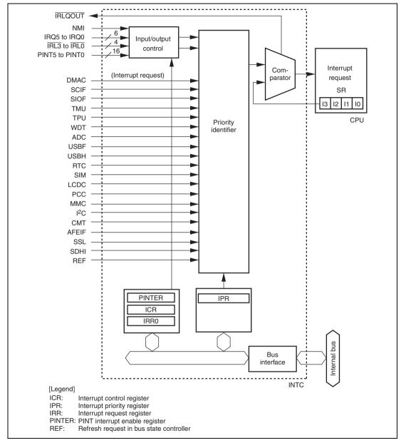
Figure 8.1 Block Diagram of INTC
