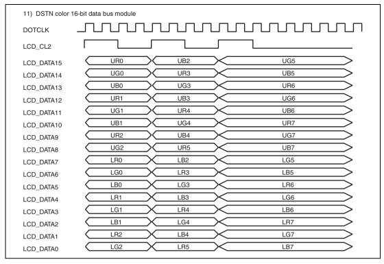
Figure 26.20 Clock and LCD Data Signal Example (DSTN Color 16-Bit Data Bus Module)
