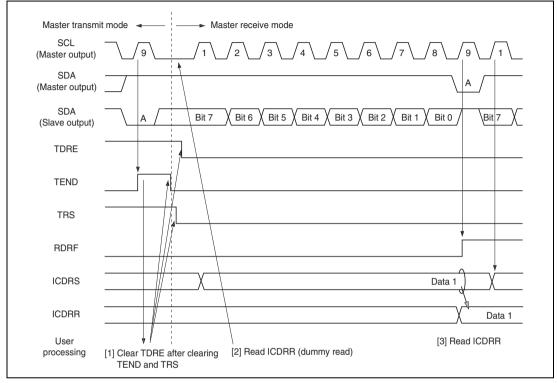
Figure 20.7 Master Receive Mode Operation Timing (1)
