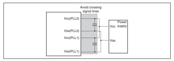
Figure 11.3 Points for Attention when Using PLL Oscillator Circuit
