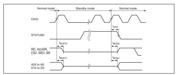
Figure 38.11 Pin Drive Timing at Standby
