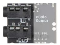
The audio output is designed for amplified devices only. This means that any attempt to use the Spectacle Audio Board with headphones or unamplified speakers will fail to produce audible output. SparkFun sells a small, amplified, rechargeable speaker which is specifically intended for use with the Spectacle Audio Board.
