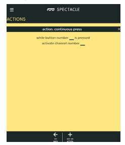
Trigger an event as soon as a button is pressed, then continue to trigger that event as long as the button is held down.
