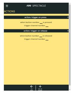
Here are the settings you'll want to put into place for this project. You can see that the "Action on Press" is tied to channel 0, and we're using button 8 (the onboard button) as the input signal. "Action on Release" is tied to channel 1, and also to button 8.
