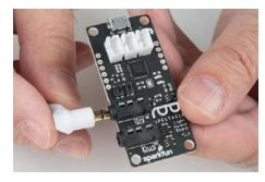
Connect the light strip adapter cable to the Light Board.
