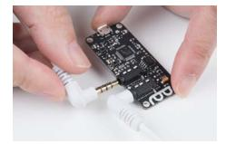
Take the other end of this cable and plug it into the audio jack of the phone, tablet, or computer that you'll be using to program the system.
