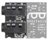
The Light Board supports up to three strands of addressable LEDs. Each strand can have up to 60 individual pixels. **Not all types of addressable LEDs are compatible with the Spectacle Light Board.** If you have questions about whether or not a particular type of LED strip is compatible with the Light Board, contact SparkFun technical support.
