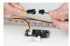
Finally, plug the Micro B end of the USB cable into the Director Board and the other end into the power adapter. Plug the power adapter into the wall. You should see one solid light and one blinking light on the Light Board, the Audio Board, and the Button Board. On the Director Board, you'll see one solid light and one light which blinks one time, then pauses, then repeats. This shows that power is present and the boards are up and running.
