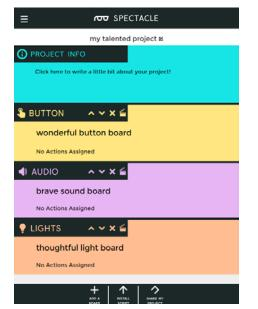
Now you'll need to add actions to each board, to tell the Spectacle system what sort of behavior you want. Click on the clapboard icon (highlighted above) for the Button Board to pull up the "Edit actions" frame.
