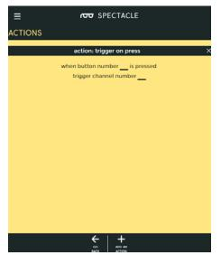
Trigger an action when a button is first pressed, regardless of how long it is subsequently held down.
