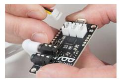
Connect the other end of the adapter cable to the light strip.
