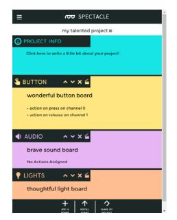
Now, add a "Play Sound" action to the Audio Board. It's the only action the Audio Board supports. Fill in the blanks on the play sound page as shown above.
