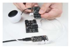
Insert the micro SD card into the Audio Board.
