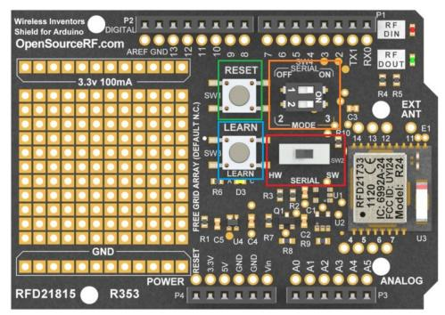
Reset Button (SW1): This is tied to the Arduino and will reset the Arduino system
