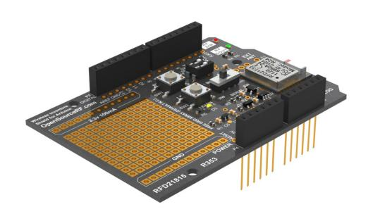
The inventors shield uses a **wireless pipe**, which is a special wireless RF module that allows you to easily and reliably, send and receive error-free wireless data between two or more Arduino boards. The inventors shield "Just Works", no complicated channels to select, to setup or initialization. Just plug it in and its ready to go. No extra libraries are required.
