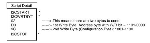
**Note:** All 6 parameters above must be listed in the same order as shown here. The parameters above with \* are not modifiable.
