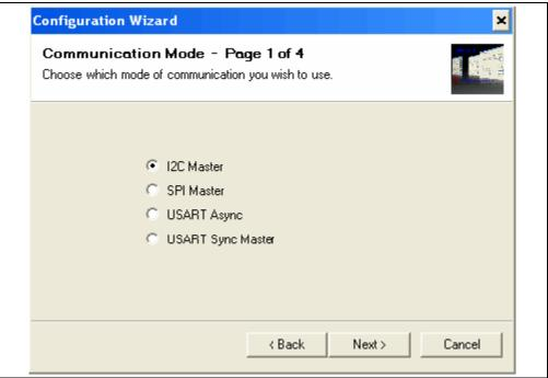
FIGURE 1-4: Step 1 - Communication Mode Selection.
