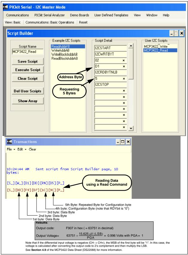
**FIGURE 1-14:** Reading Conversion Results. Note that the Input = 0.996V is applied at Ch.1. The reading indicates the measured value is 0.996 Volts.
