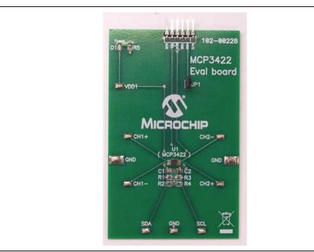
FIGURE 1-1: Front View of the MCP3422 Evaluation Board.
