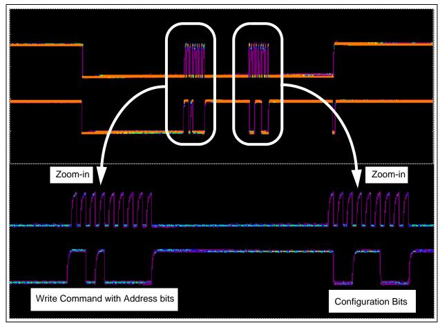
**FIGURE 1-12:** I<sup>2</sup>C Write Command Waveforms for the MCP3422.
