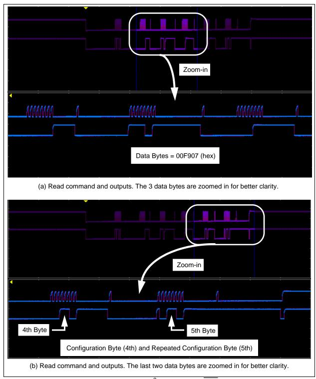
**FIGURE 1-15:** Read Command and Data on  $l^2C$  bus. Note the  $\overline{RDY}$  bit in 4th byte is "0". This means the conversion data just read is the latest conversion data. The  $\overline{RDY}$  bit becomes "1" in the 5th byte (repeated byte). This means the device is now in the process of new conversion and the new result is not ready yet.
