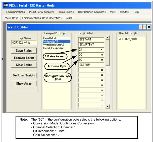
FIGURE 1-11: Script File Example for the I<sup>2</sup>C Write Command.
