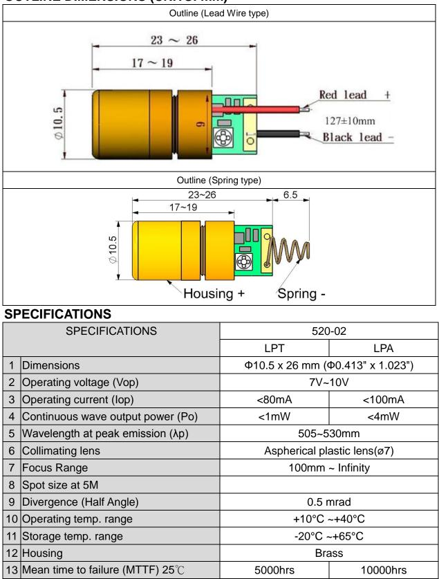
Note : Laser module housing is an electrical positive surface, it is imperative that contact between the laser module
