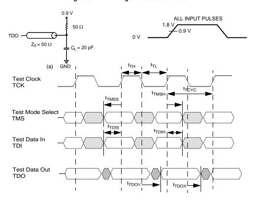
Note 19. Test conditions are specified using the load in TAP AC Test Conditions.  $t_R/t_F=1$  ns.
