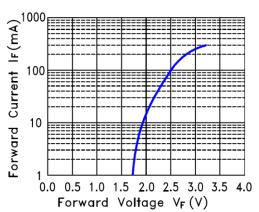
Fig.3 Forward Current vs. Forward Voltage
