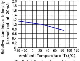
Fig.5 Relative Luminous Intensity VS. Ambient Temperature
