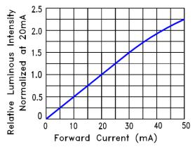
Fig.4 Relative Luminous Intensity vs. Forward Current
