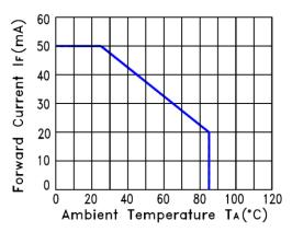
Fig.2 Forward Current Derating Curve
