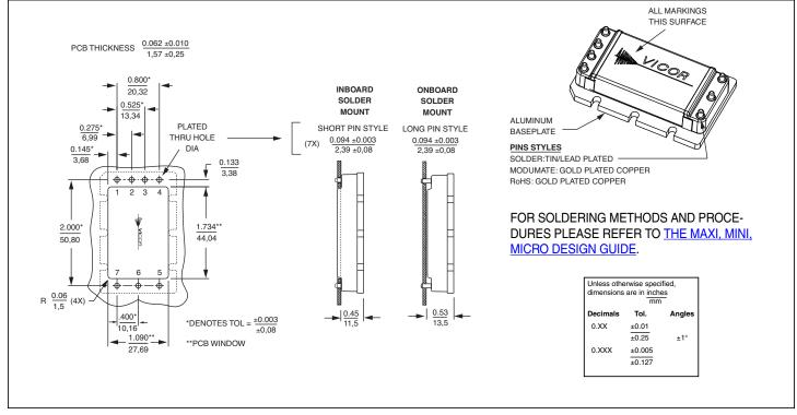
Figure 14 — PCB mounting specifications
