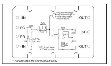
Figure 3 — PC/SC module alarm logic.
