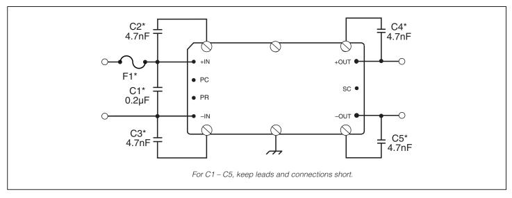
*Figure 1* — *Basic module operation requires fusing, grounding, bypassing capacitors.* \* *See Maxi, Mini, Micro Design Guide.*
