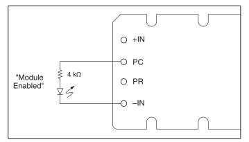
Figure 4 — LED on-state indicator.
