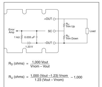
Figure 8 — Output voltage trim down and trim up circuit.
