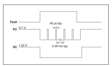
Figure 5 — PC/SC module alarm timing.
