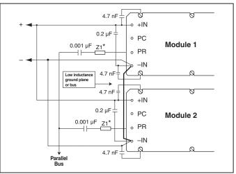
*Figure 9* — *AC* coupled single-wire interface. \* See Maxi, Mini, Micro Design Guide.
