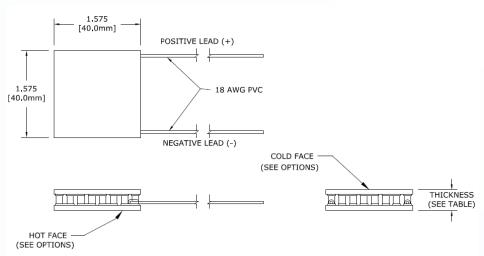
Ceramic Material: Alumina ( $Al_2O_3$ ) Solder Construction: 138°C, Bismuth Tin (BiSn)
