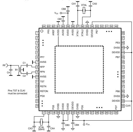
The power supply bypass capacitors (CB2, CB4) are connected to the external analog supply pin (EVDD, pin 59) and external digital supply pin (DEVDD, pin 23). Pins 34, 44 and 54 supply the digital port pins.
