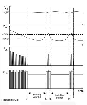
Figure 41. Waveforms of Burst Operation
