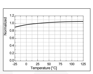
Figure 20. Feedback Source Current (I<sub>FB</sub>) vs. T<sub>A</sub>
