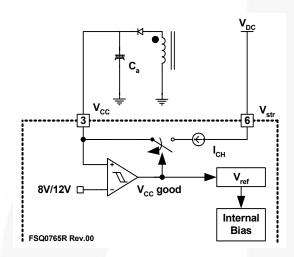
Figure 31. Startup Circuit
