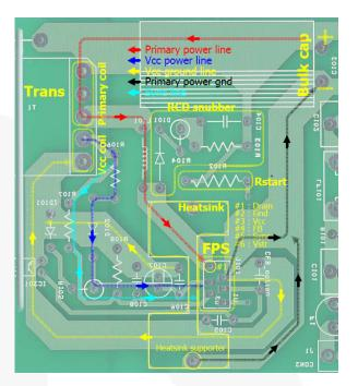
Figure 45. Recommended PCB Layout
