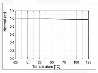
Figure 22. Burst-Mode High Threshold Voltage (V<sub>burh</sub>) vs. T<sub>A</sub>
