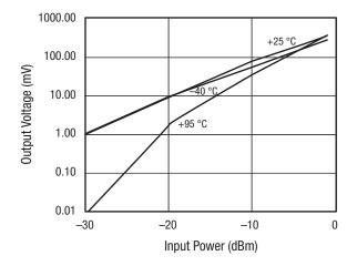
Figure 5. Output Voltage vs Input Power Over Temperature (Load Resistance = 1 k $\Omega$ )
