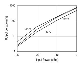
Figure 7. Output Voltage vs Input Power Over Temperature (Load Resistance =  $100 \text{ k}\Omega$ )
