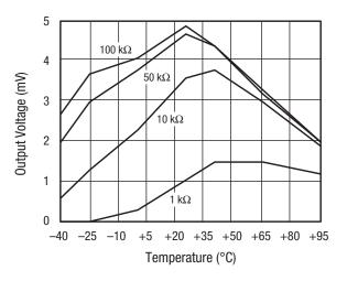
Figure 8. Output Voltage vs Temperature Over Load Resistance @ -30 dBm
