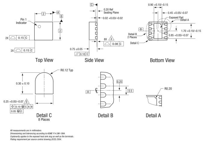
Dimension applies to metalized terminal and is measured between 0.15 mm and 0.30 mm from terminal tip.
