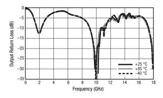
Figure 9. Broadband Output Return Loss vs Frequency
