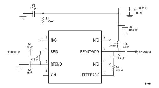
Figure 16. SKY67100-396LF Evaluation Board Schematic
