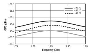
Figure 12. OIP3 vs Frequency (PIN = -20 dBm, Spacing = 5 MHz)
