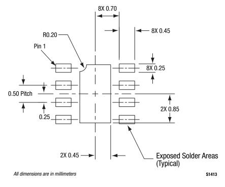
Figure 17. SKY67100-396LF PCB Layout Footprint (Top View)
