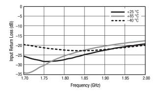
Figure 6. Narrowband Input Return Loss vs Frequency
