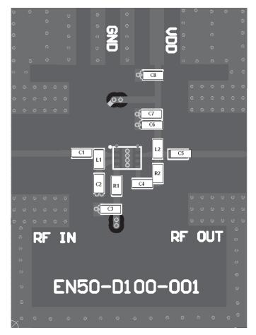
Figure 15. SKY67100-396LF Evaluation Board Assembly Diagram
