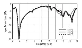
Figure 5. Broadband Input Return Loss vs Frequency
