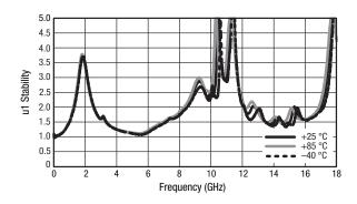
Figure 13. u1 Stability vs Frequency
