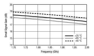
Figure 4. Narrowband Gain Response vs Frequency
