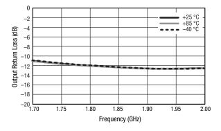
Figure 10. Narrowband Output Return Loss vs Frequency
