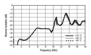
Figure 7. Broadband Reverse Isolation vs Frequency
