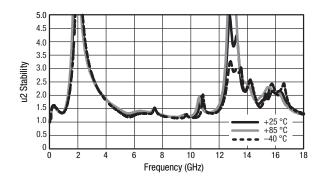
Figure 14. u2 Stability vs Frequency
