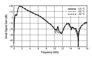
Figure 3. Broadband Gain Response vs Frequency
