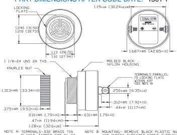
NOTE A: TERMINALS-032 BRASS TIN PLATED, TAPPED FOR #6-32 SCREW, TWO #6-32 NICKEL PLATED BRASS SCREWS INCLUDED, WILL ACCEPT 1/4\* OUICK CONNECT. NOTE B: MOUNTING- REMOVE BLACK PLASTIC NUT AND INSERT THREADED FRONT THROUGH 1.25' HOLE PUNCHED IN PANEL, IF DRIENTATION IS NEEDED, NOTE LOCKING FLATS ON DRAWING, SCREW NUT BACK ON. DO NOT OVERTIGHTEN.
