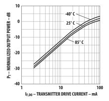
Figure 2. Typical normalized optical power vs. drive current
