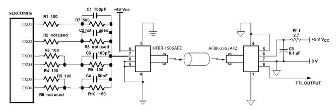
Figure 5. Recommended drive circuit according to SERCOS An17 (Ifnom ~ 35 mA) for data rate up to 16 MBd with transmitter HFBR-1506AFZ
