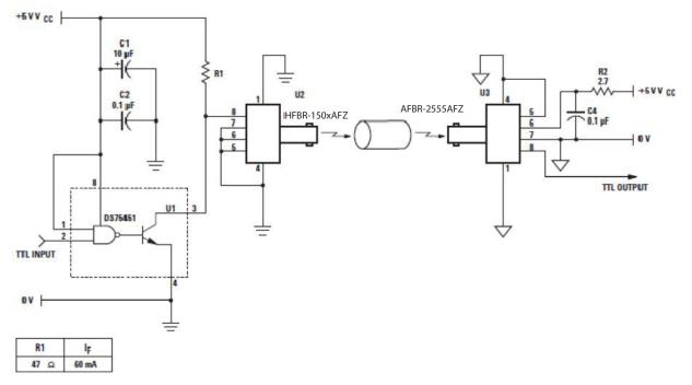
Figure 4. Recommended transmitter and receiver drive circuit ( $I_{F, on} = 60$  mA nominal at  $T_A = 25^{\circ}$  C) for data rate up to 10 MBd, with transmitter HFBR-1505AFZ
