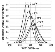
Figure 3. Typical normalized optical spectra
