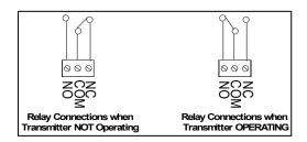
The action of the relay outputs is set by the Option link setting Jumper. A link is made / removed by the small shorting link 'cap' placed over the pin header.
