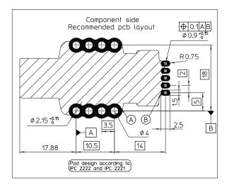
(Layout example with 4 jumpers in parallel)
