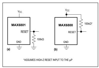
Figure 2. Ensuring Reset Valid Down to  $V_{CC} = 0V$
