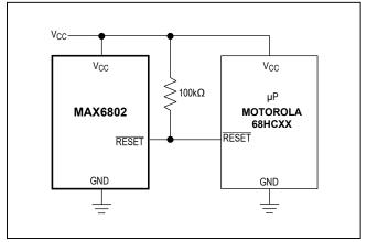
Figure 1. Interfacing to μPs with Bidirectional Reset Pins
