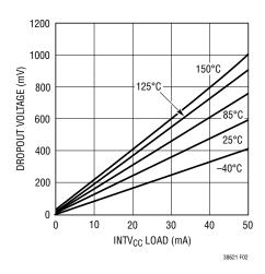
Figure 2. INTV<sub>CC</sub> LDO Dropout Voltage vs Current
