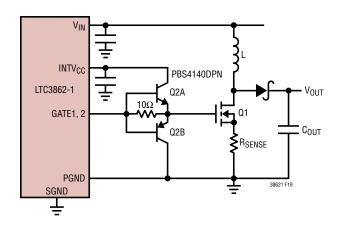
Figure 19. External Buffer Circuit
