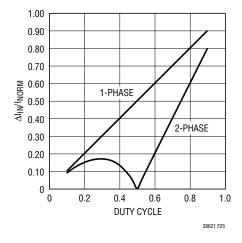
Figure 25. Normalized Input Peak-to-Peak Ripple Current
