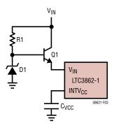
Figure 3. Using the LTC3862-1 with an External Bias Supply
