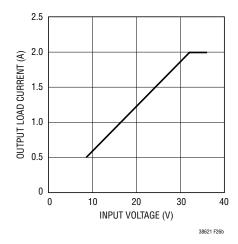
Figure 26b. Output Current vs Input Voltage
