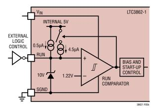
Figure 5b. On/Off Control Using External Logic
