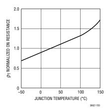
Figure 20. Normalized Power MOSFET R<sub>DS(ON)</sub> vs Temperature
