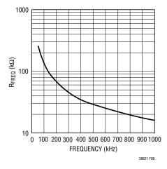
Figure 6. FREQ Pin Resistor Value vs Frequency
