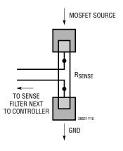
Figure 16. Connecting the SENSE<sup>+</sup> and SENSE<sup>-</sup> Traces to the Sense Resistor Using a Kelvin Connection
