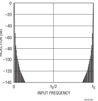
Figure 31. Rejection vs Frequency at  $V_{\text{IN}}$
