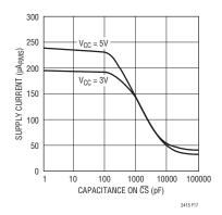
Figure 17. CS Capacitance vs Supply Current
