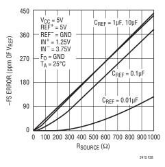
Figure 28. –FS Error vs  $R_{SOURCE}$  at REF<sup>+</sup> and REF<sup>-</sup> (Large  $C_{REF}$ ).
