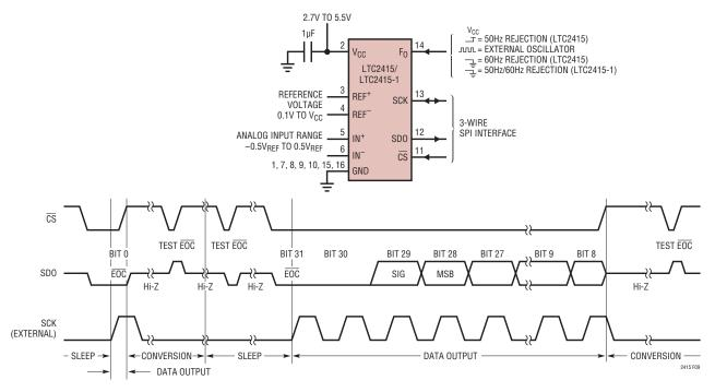
Figure 9. External Serial Clock, Reduced Data Output Length
