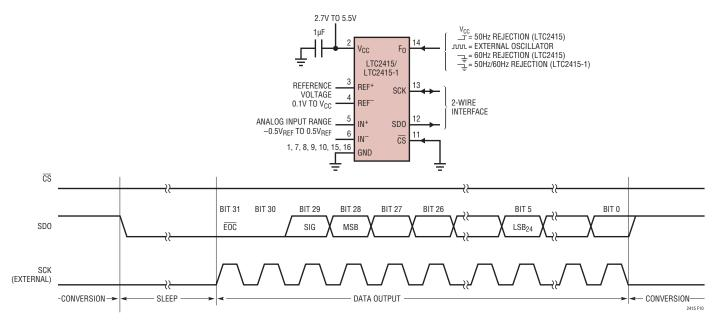
Figure 10. External Serial Clock,  $\overline{CS} = 0$  Operation (2-Wire)
