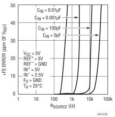
Figure 20. +FS Error vs  $R_{SOURCE}$  at IN<sup>+</sup> or IN<sup>-</sup> (Small C<sub>IN</sub>)
