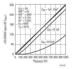
Figure 22. +FS Error vs R<sub>SOURCE</sub> at IN<sup>+</sup> or IN<sup>-</sup> (Large C<sub>IN</sub>)
