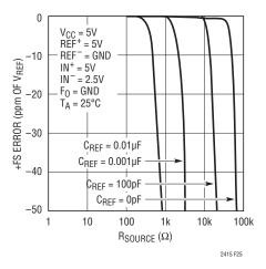
Figure 25. +FS Error vs  $R_{SOURCE}$  at REF<sup>+</sup> or REF<sup>-</sup> (Small C<sub>IN</sub>)
