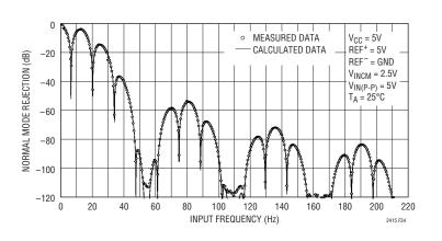
Figure 34. Input Normal Mode Rejection vs Input Frequency with Input Perturbation of 100% of Full Scale
