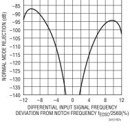
Figure 7c. LTC2415/LTC2415-1 Normal Mode Rejection When Using an External Oscillator of Frequency f<sub>EOSC</sub> with Running Averages
