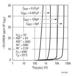
Figure 26. -FS Error vs R<sub>SOURCE</sub> at REF<sup>+</sup> or REF<sup>-</sup> (Small C<sub>IN</sub>)
