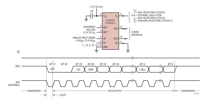
Figure 13. Internal Serial Clock, Continuous Operation
