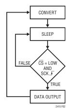
Figure 2. LTC2415 State Transition Diagram
