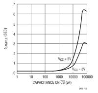
Figure 15.  $\overline{\text{CS}}$  Capacitance vs  $t_{\text{SAMPLE}}$
