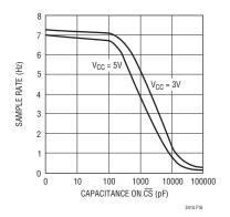
Figure 16. CS Capacitance vs Output Rate
