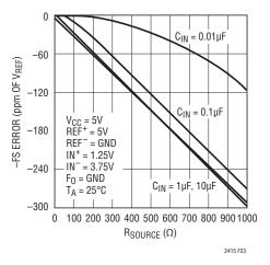
Figure 23. –FS Error vs  $R_{SOURCE}$  at  $IN^{+}$  or  $IN^{-}$  (Large  $C_{IN})$
