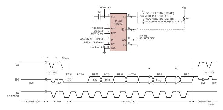
Figure 11. Internal Serial Clock, Single Cycle Operation
