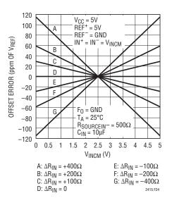
Figure 24. Offset Error vs Common Mode Voltage ( $V_{INCM} = IN^+ = IN^-$ ) and Input Source Resistance Imbalance ( $\Delta R_{IN} = R_{SOURCEIN} + - R_{SOURCEIN}$ ) for Large C<sub>IN</sub> Values ( $C_{IN} \ge 1\mu F$ )
