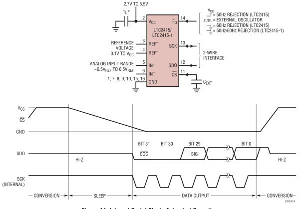
Figure 14. Internal Serial Clock, Auto-start Operation
