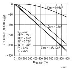
Figure 27. +FS Error vs  $R_{SOURCE}$  at REF<sup>+</sup> and REF<sup>-</sup> (Large  $C_{REF}$ )
