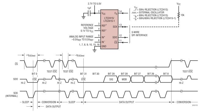
Figure 12. Internal Serial Clock, Reduced Data Output Length
