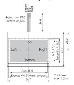
connecting a voltage of e.g. 3.3V to the pins *Top-Bottom* makes it possible to read out a voltage on pin *Left* or *Right* which is linear to the Y-coordinate of the pressed point. The X-coordinate will result when the voltage will be supplied to *Left-Right* and measurement is done at *Top* or *Bottom*.
