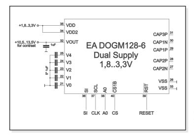
If an external source of  $+10.5 \sim +13.5V$  (does not have to be stabilized) is available, the charge pump is not needed and less external components are required.
