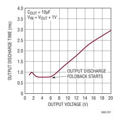
Figure 7. Discharge Time vs Output Voltage
