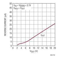
Figure 8. LT3063 Reverse Output Current
