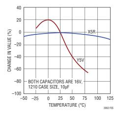
Figure 5. Ceramic Capacitor Temperature Characteristics
