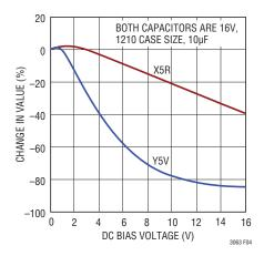
Figure 4. Ceramic Capacitor DC Bias Characteristics
