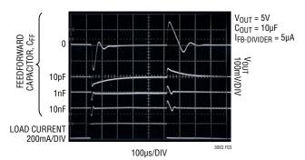
Figure 3. Transient Response vs Feedforward Capacitor
