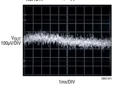
$C_{OUT} = 10 \mu F$  $I_{LOAD} = 200 \text{mA}$
