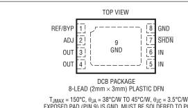
$T_{JMAX}$  = 150°C,  $\theta_{JA}$  = 38°C/W TO 45°C/W,  $\theta_{JC}$  = 3.5°C/W EXPOSED PAD (PIN 9) IS GND, MUST BE SOLDERED TO PCB
