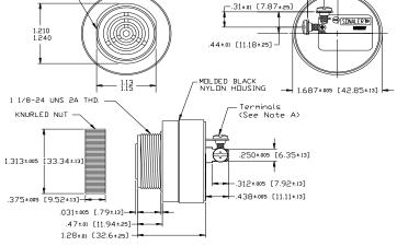
NOTE A: TERMINALS-.032 BRASS TIN PLATED, TAPPED FOR #6-32 SCREW. TWO #6-32 NICKEL PLATED BRASS SCREWS INCLUDED. WILL ACCEPT 1/4" OUICK CONNECT.
