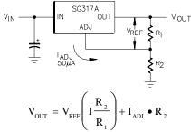
Figure 17 – Basic Regulator Circuit
