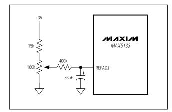
Figure 3b. MAX5133 Reference Adjust Circuit
