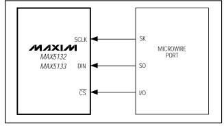
Figure 5. MICROWIRE Interface Connections
