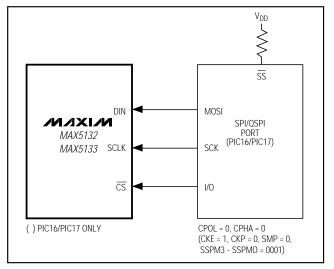
Figure 4. SPI/QSPI Interface Connections (PIC16/PIC17)
