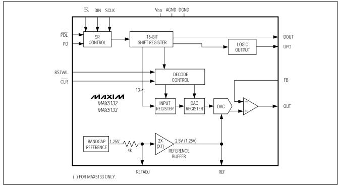
Figure 1. Simplified Functional Diagram
