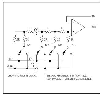
Figure 2. Simplified Inverted R-2R DAC Structure
