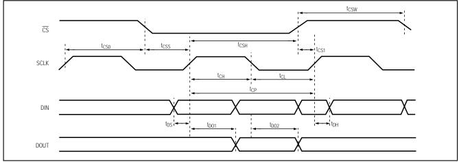
Figure 7. Detailed Serial-Interface Timing
