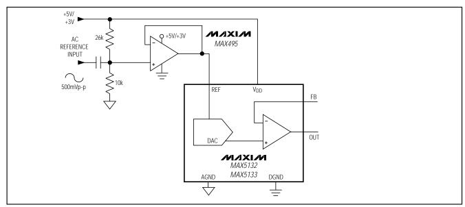
Figure 13. External Reference with AC Components
