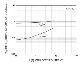
Figure 2. Saturation Voltage
