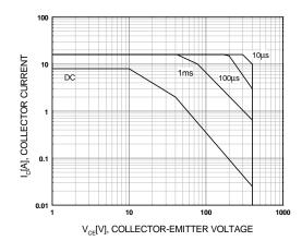
Figure 6. Forward Biased Safe Operating Area
