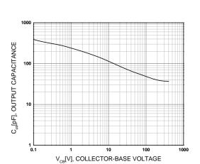
Figure 3. Collector Output Capacitance
