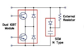
Figure 1 Style SCM Discharge restrictive decoupling used to protect dual IGBT modules
