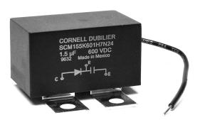
Use style SCM as a discharge restrictive de-coupling to protect dual IGBT modules from overvoltage, Figure 1. Style SCM may also be used as an "N" or "P" type snubber component for a clamp snubber where single IGBT modules are used, figure 2.
