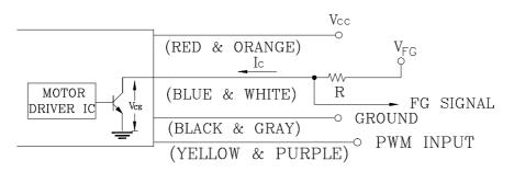
CAUTION: THE FG SIGNAL LEAD WIRE MUST BE KEPT AWAY FROM "+" LEAD WIRE & "-" LEAD WIRE.
