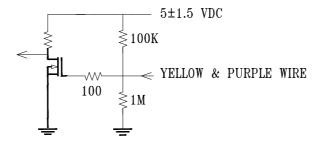
13-1. THE FAN SPEED WILL DEFAULT TO MAXIMUM WHEN THE SPEED CONTROL INPUT IS LEFT UNCONNECTED.
