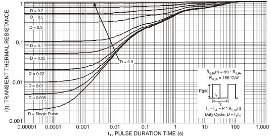
Figure 3 Transient Thermal Response
