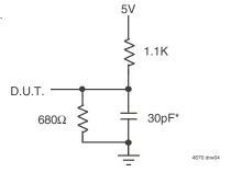
Figure 2. Output Load
