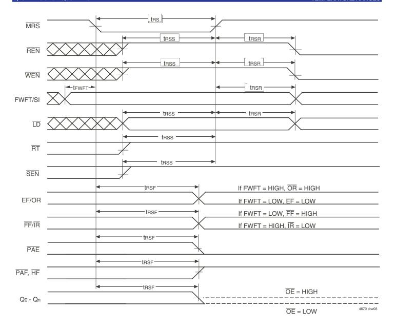
Figure 5. Master Reset Timing
