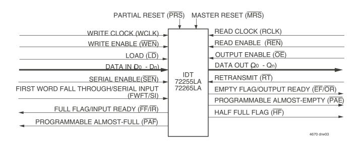
Figure 1. Block Diagram of Single 8,192 x 18 and 16,384 x 18 Synchronous FIFO
