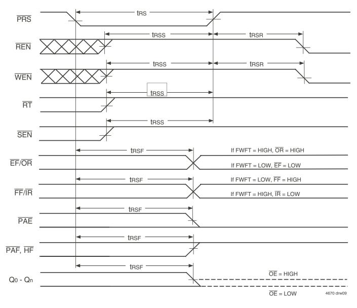
Figure 6. Partial Reset Timing
