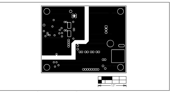
Figure 5. MAX5069A EV Kit PC Board Layout—Inner Layer, GND Plane
