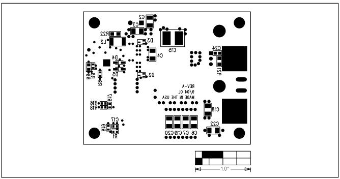
Figure 8. MAX5069A EV Kit Component Placement Guide—Solder Side
