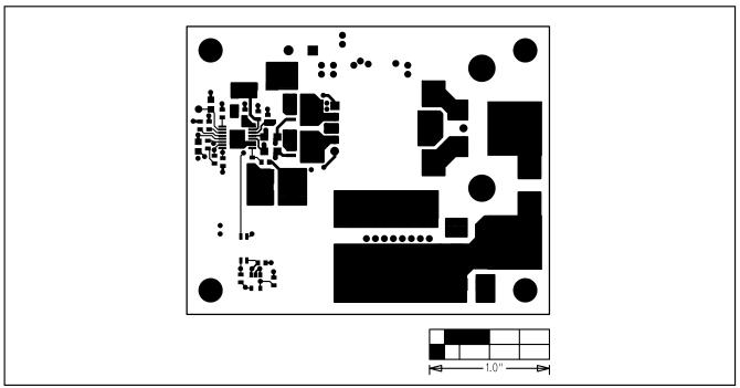
Figure 4. MAX5069A EV Kit PC Board Layout—Component Side
