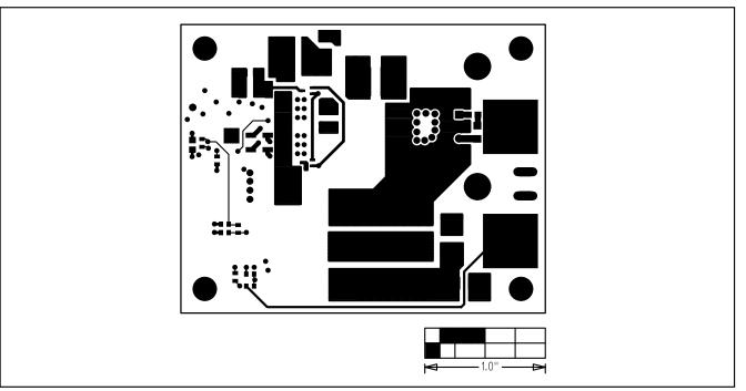
Figure 7. MAX5069A EV Kit PC Board Layout—Solder Side
