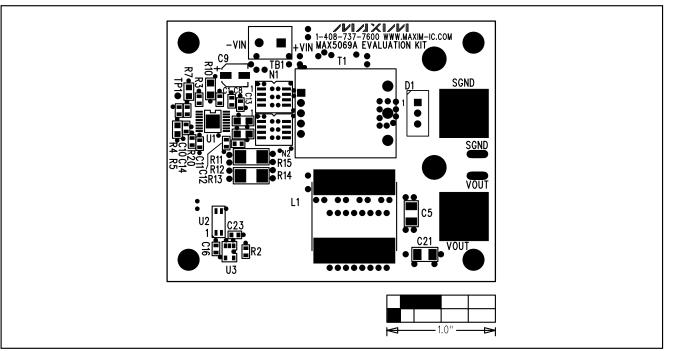
Figure 3. MAX5069A EV Kit Component Placement Guide—Component Side
