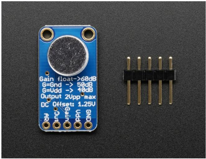
This fancy microphone amplifier module is a step above the rest, with built in automatic gain control. The AGC in the amplifier means that nearby 'loud' sounds will be quieted so they don't overwhelm & 'clip' the amplifier, and even quiet, far-away sounds will be amplified. This amplifier is great for when you want to record or detect audio in a setting where levels change and you don't want to have to tweak the amplifier gain all the time.
