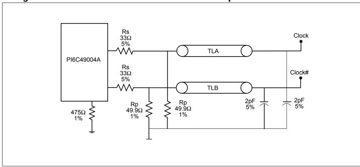
Figure 4. Configuration Test Load Board Termination
