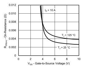
On-Resistance vs. Gate-to-Source Voltage
