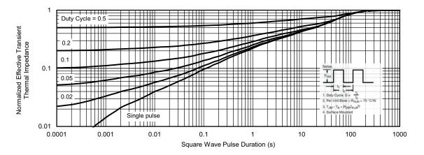
Normalized Thermal Transient Impedance, Junction-to-Ambient
