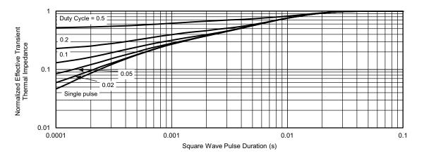
Normalized Thermal Transient Impedance, Junction-to-Case
