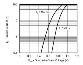
Source-Drain Diode Forward Voltage
