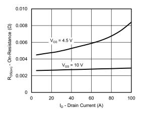
On-Resistance vs. Drain Current
