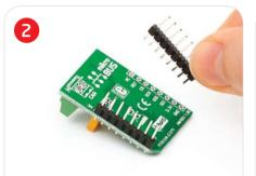
Turn the board upside down, so that bottom side is facing you upwards. Place shorter parts of the header pins in the both soldering pad locations.
