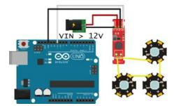
If you have more than a couple of LEDs, you should provide an independent power supply from the Arduino. Multiple LEDs can be connected in series, as shown, and the supply voltage should be at least 2-3V higher than the sum of the forward voltages of the LEDs.
