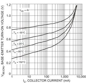
Figure 3 Typical Base-Emitter Turn-On Voltage vs. Collector Current
