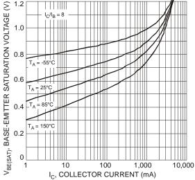
Figure 4 Typical Base-Emitter Saturation Voltage vs. Collector Current
