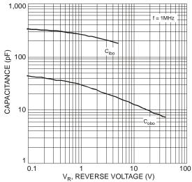
Figure 5 Typical Capacitance Characteristics
