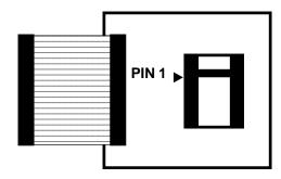
NOTE: Align PIN 1 of 18 pin devices with the arrow indicated.
